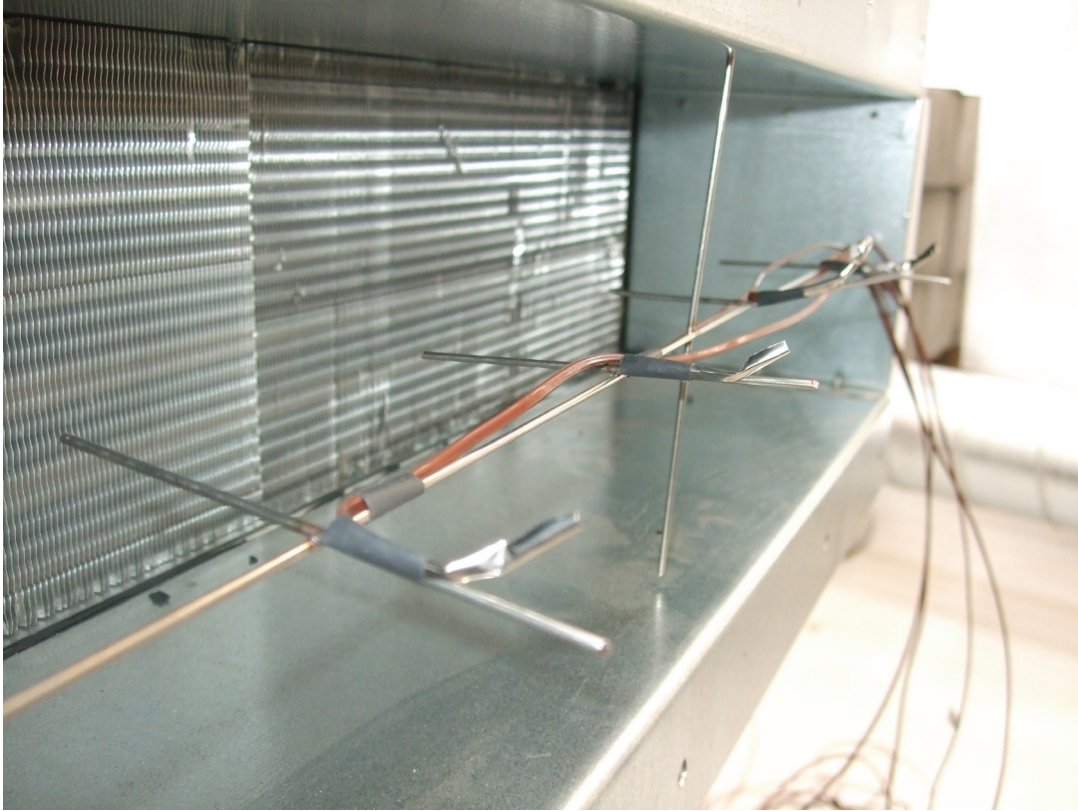
Figure 25: Picture of thermocouple installation at heat exchanger inlet, complete with radiation heat shielding.
