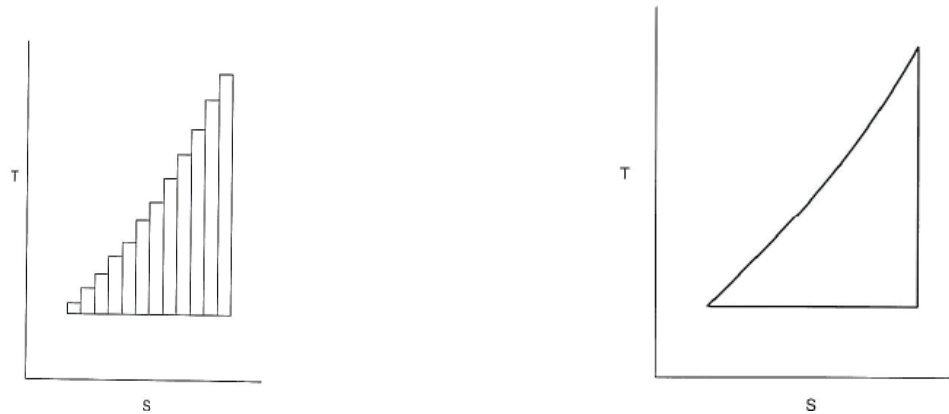
Figure 14: The ideal trilateral cycle; as a composition of infinitesimal Carnot cycles (left) and on integral form (right) [16]
