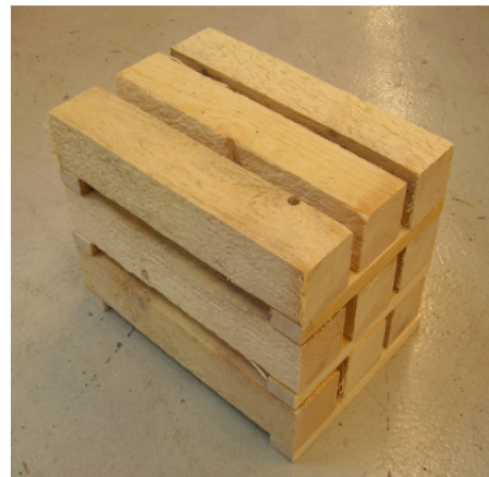
Figure 6.7: Size of the standard test fuel
