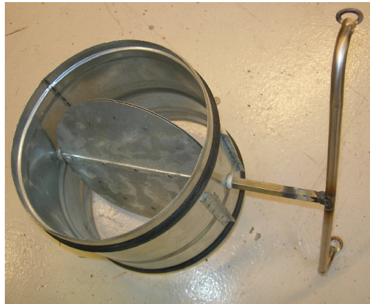
Figure 6.8: Damper used during EN-13240 tests
