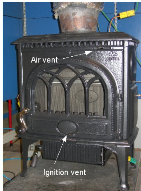
Figure 5.3: Front view of Jøtul F3 with both air vents
