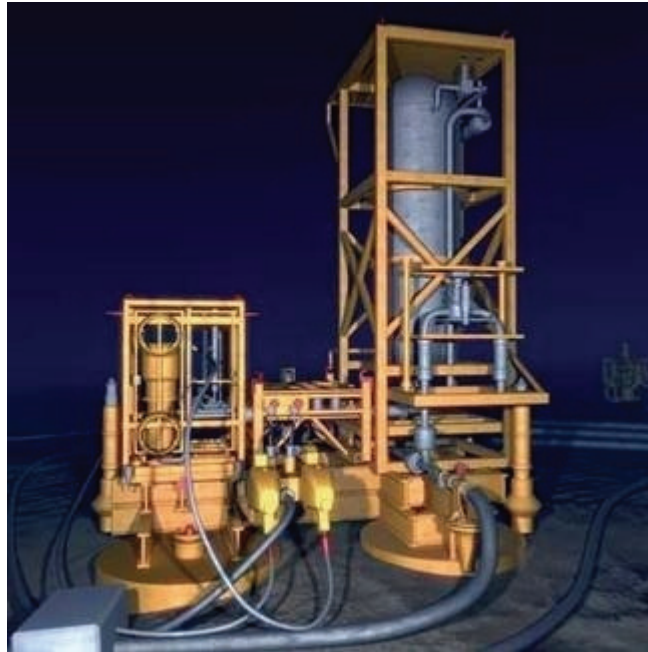
Figure 2-17: The SSU with vertical separator and two hybrid pumps [30]
