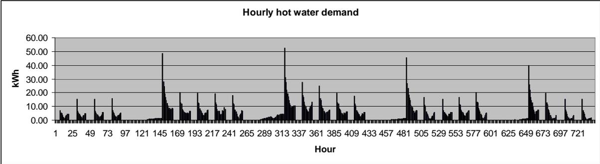
Figure 32. Case 2; hourly hot water demand in January. The graph shows how very high demands for heating occur early in the morning. Total hot water supply for January is 2758.8 kWh.
