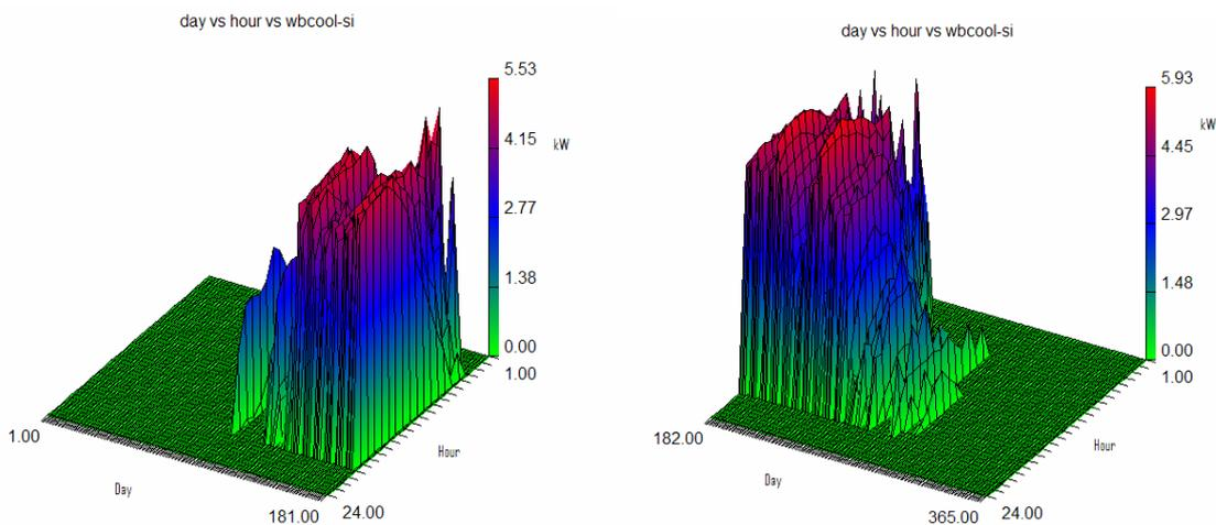
Figure 35. Case 1. Cold water demand for an entire year. Case 1. Day vs. Hour vs. whole building cooling in SI-units. [Appendix F]
