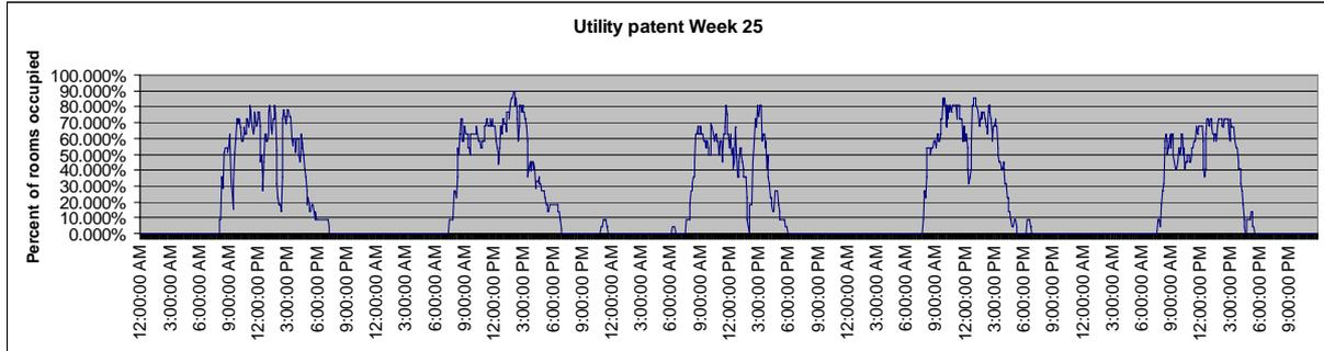
**Figure 3. Measured data for five working days in week 25. From June 18<sup>th</sup> to June 22<sup>nd</sup>. Calculated using the average of SWE-V, SWE and MIM sensors.**
