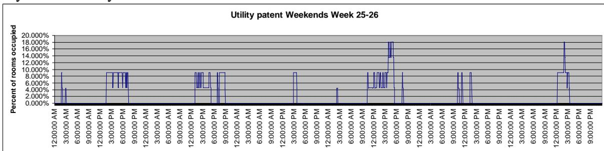
**Figure 4. Measured data for two weekends in week 25 and 26. Max value 18% occupancy. Calculated using the average of SWE-V, SWE and MIM sensors. Note that the y-axis only reaches 20%.**
