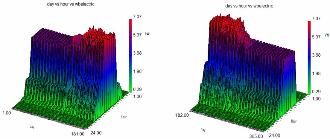
**Figure 44. Case 2. Electric demand for an entire year. Day vs. Hour vs. whole building electric in SI-units. Note how the pattern changes for months with cooling demand. [Appendix I]**
