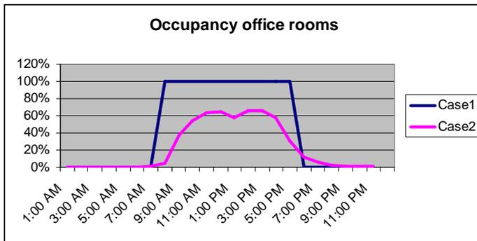
**Figure 28. Minimum ventilation rate as a percentage of the zones ventilation capacity. Case 2 line represents the occupancy in the office zones based on the results from chapter 0**
