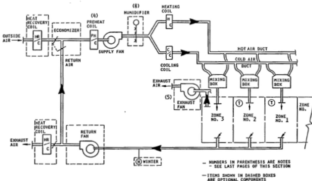
Figure 16 Air mixing system (DDS, Dual-Duct System) [8]
