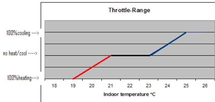
**Figure 19. Throttling-range for the cantina HVAC system**
