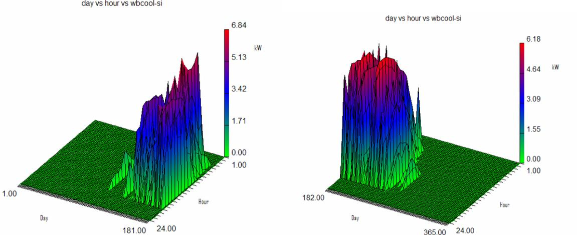
Figure 42. Case 2. Cold water demand for an entire year. Day vs. Hour vs. whole building cooling in SI-units. [Appendix H]
