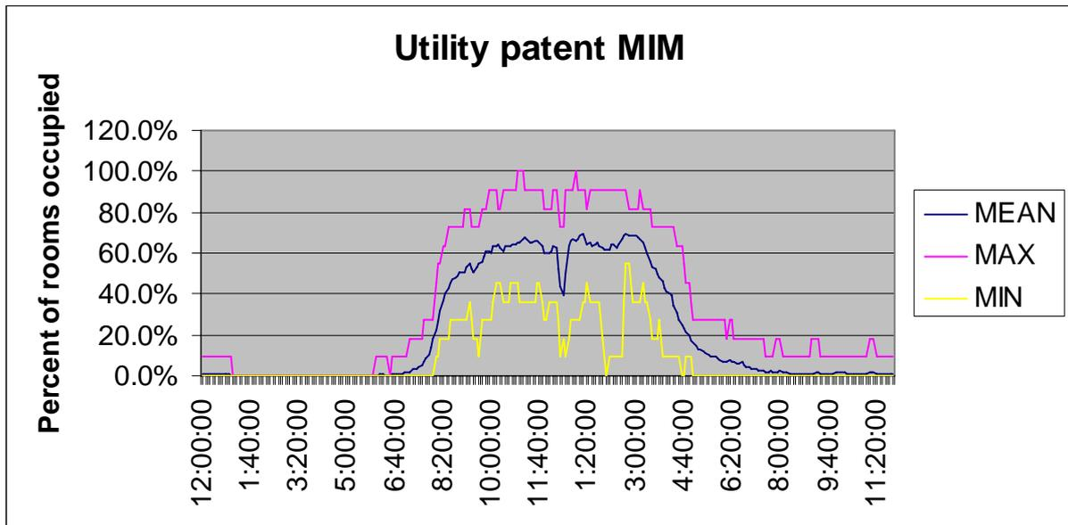
**Figure 9.** Max, min and average occupancy based on twenty nine working days. Calculated using the data from MIM sensors only.
