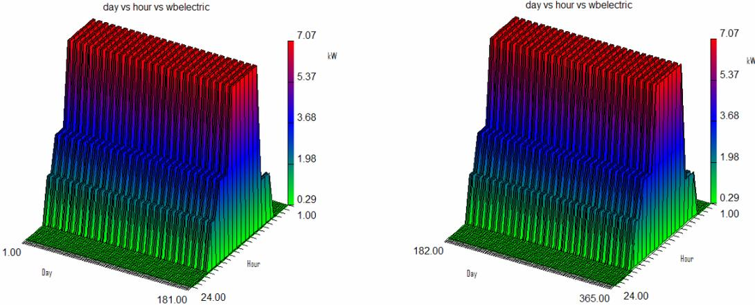
**Figure 39. Case 1. Electric demand for an entire year. Day vs. Hour vs. whole building electric in SI-units. Note the repetitive pattern.**
