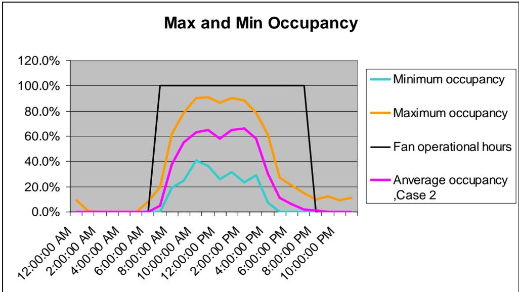
**Figure 47. Maximum and minimum occupancy. The values are based on the experiment with infrared motion sensors, average occupancy for all offices. Same values as presented in chapter 1.2.**
