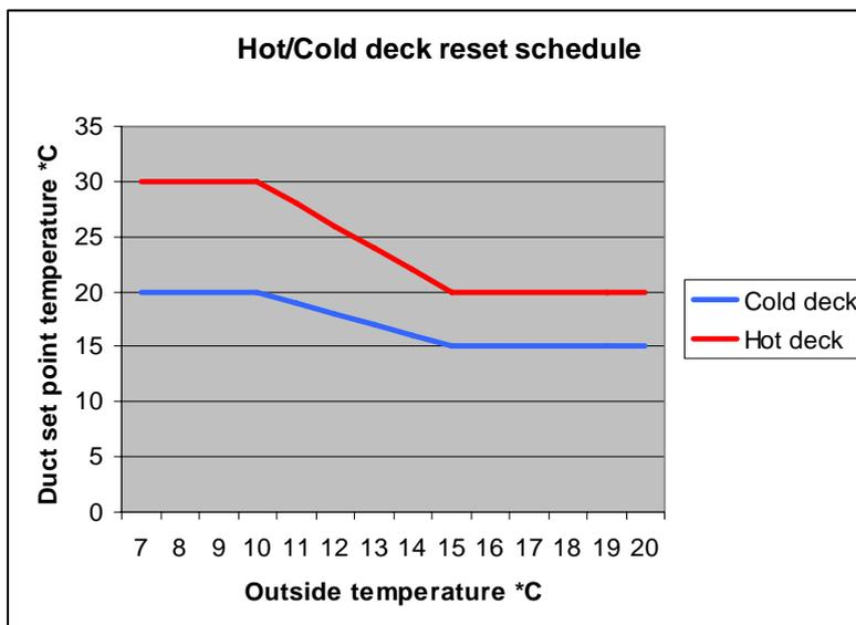
Figure 24. Hot and Cold deck reset schedule based on outside air temperature.
