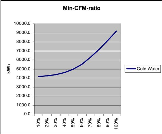
Figure 48. The affect on cold water demand when changing the minimum cfm ratio in the system terminal boxes of Case 3.
