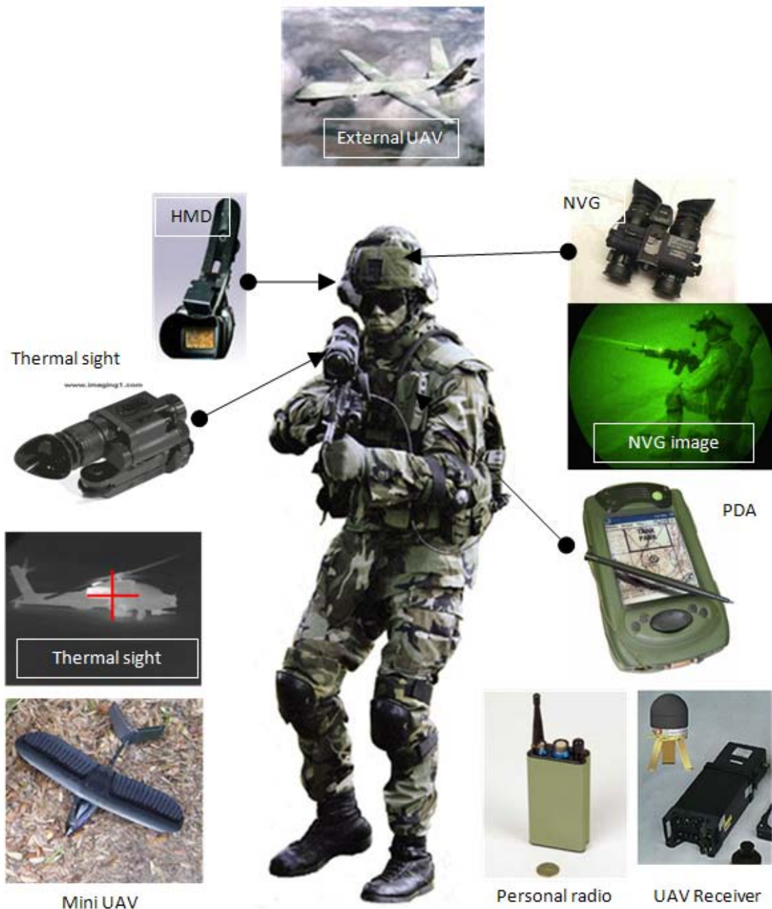
Figure 3.0 Soldiers main electrical equipment.
