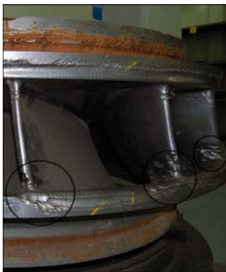
(a) Erosion at runner outlet
