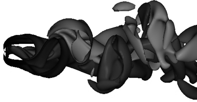
Figure 13 : Side-view of 3-dimensional Iso-surface of spanwise vorticity. The flow is from left to right. Details are the same as caption of Figure 11(b)
