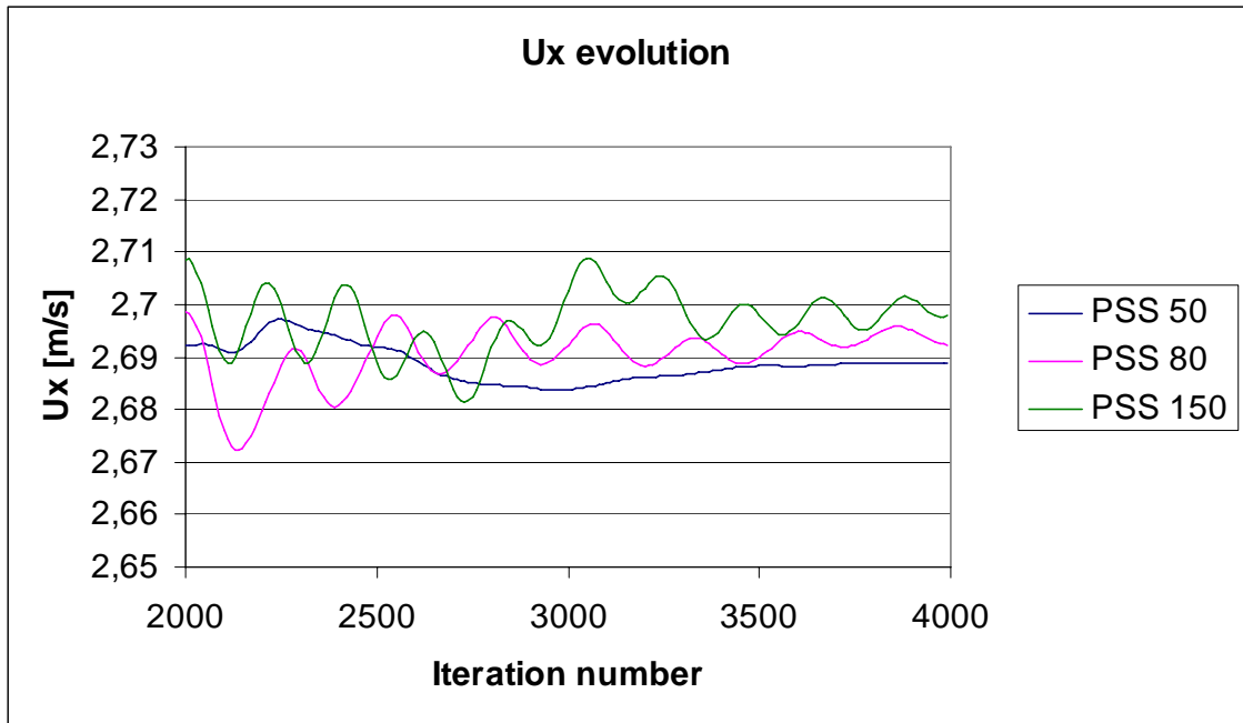
Figure 12: Close-up of Figure 11, a detailed view of the converging velocity the last 2000 iterations. The best convergence is found for the pseudo-sonic speed equal to 50m/s. Values are collected from cell number i=50 and j=12 . This is about 1 cm above ground level in the area of flow separation, 1.3cm downwind from hill summit.
