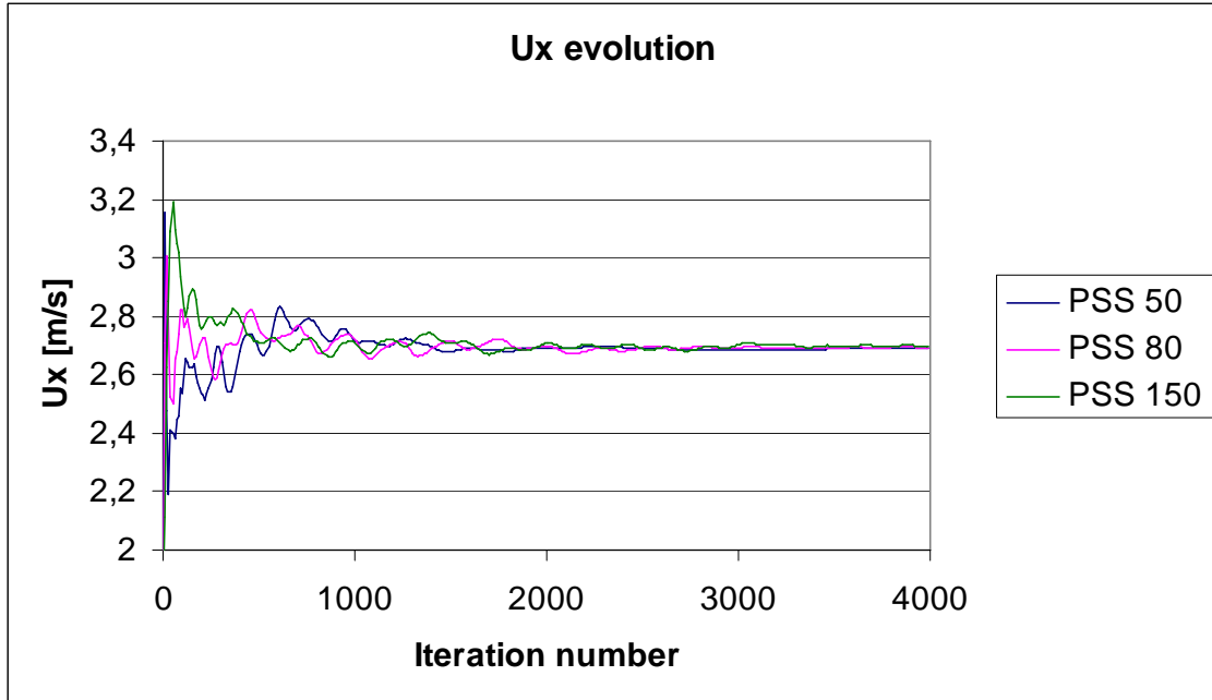
Figure 11: The convergence of velocity with the three different pseudo-sonic speeds. Sufficient convergence is found after about 4000 iterations. Values are collected from cell number i=50 and j=12 . This is about 1 cm above ground level in the area of flow separation, 1.3cm downwind from hill summit.
