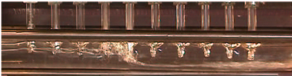
Figure 4.12: Two-phase distribution in glass manifold M12. Refrigerant flows in from the right. HFC-134a, \dot{m}_{mIn} = 0.042 kg/s, x_{mIn} = 0.2 .
