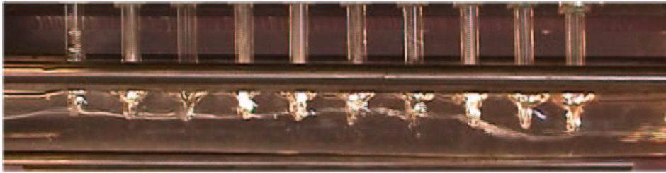
Figure 4.11: Two-phase distribution in glass manifold M12. Refrigerant flows in from the right. HFC-134a, \dot{m}_{mIn} = 0.042 kg/s, x_{mIn} = 0.05 .
