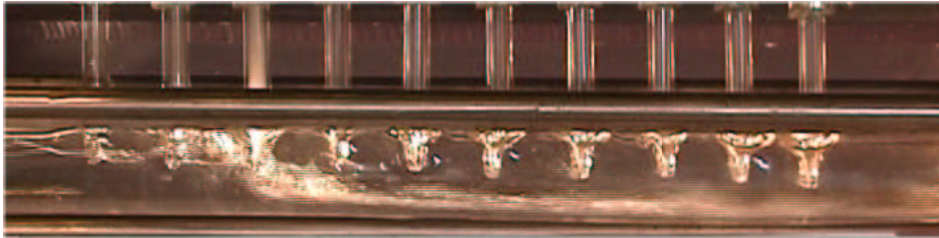
Figure 4.13: Two-phase distribution in glass manifold M12. Refrigerant flows in from the right. HFC-134a, \dot{m}_{mIn} = 0.042 \text{ kg/s} , x_{mIn} = 0.36 .
