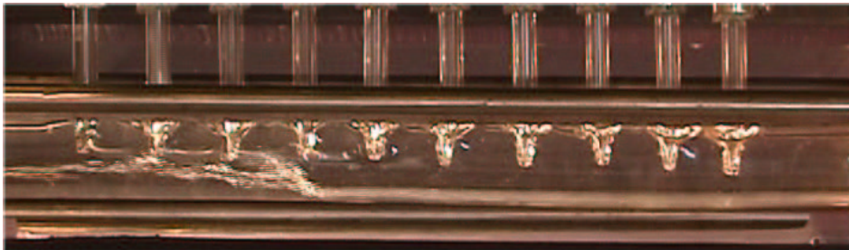
Figure 4.15: Two-phase distribution in glass manifold M12. Refrigerant flows in from the right. HFC-134a, \dot{m}_{mIn} = 0.017 \text{ kg/s} , x_{mIn} = 0.99 .
