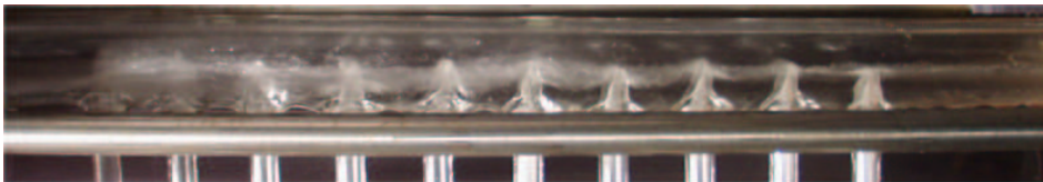
Figure 4.16: Two-phase distribution in glass manifold M12. Downward branch tubes. Refrigerant flows in from the left. HFC-134a, \dot{m}_{mIn} = 0.042 \text{ kg/s} , x_{mIn} = 0.36 .
