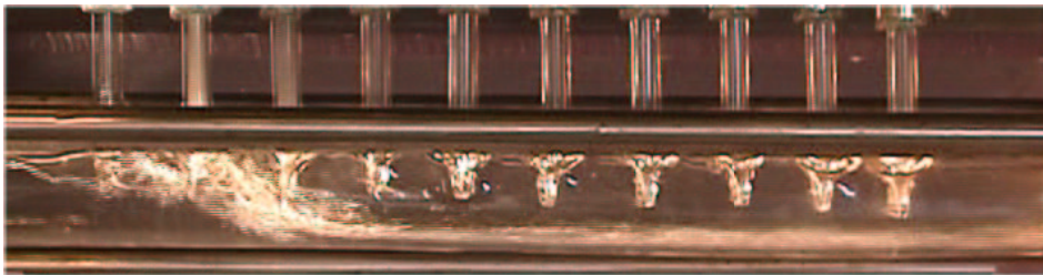
Figure 4.14: Two-phase distribution in glass manifold M12. Refrigerant flows in from the right. HFC-134a, \dot{m}_{mIn} = 0.042 \text{ kg/s} , x_{mIn} = 0.45 .
