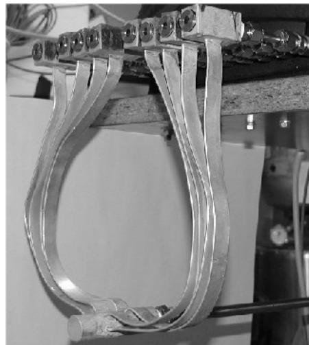
Figure 4.9: Star manifold, M11, with numbering of MPE-tubes used in the presentation of the results. Branch tubes No 1, 3, 6 and 8 constituted the first row closest to the inlet, while branch tubes No 2, 4, 5 and 7 constituted the second row.
