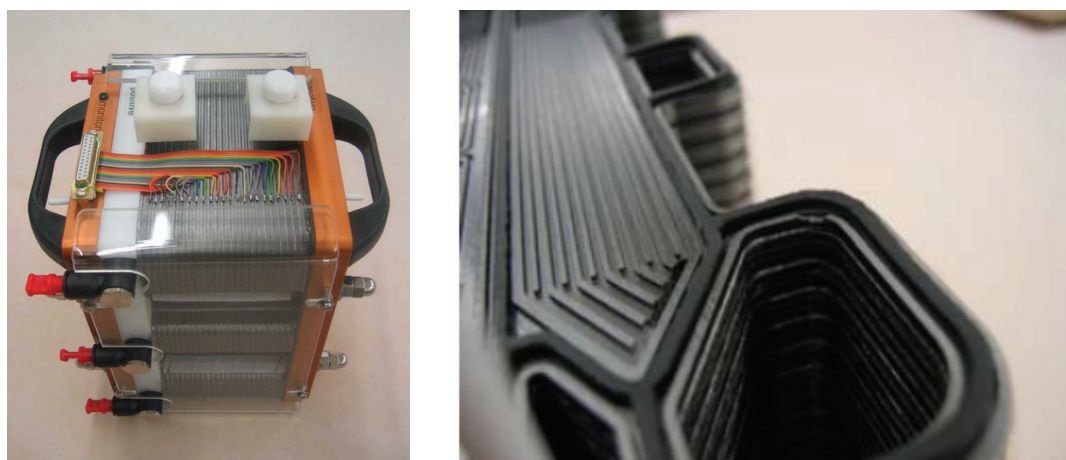
Figure 10.2: The 1.2 kW water-cooled PEM fuel cell from HTI Biel. A) The fuel cell stack. B) A detail of the internal humidification channels for inlet air on one cell plate.
