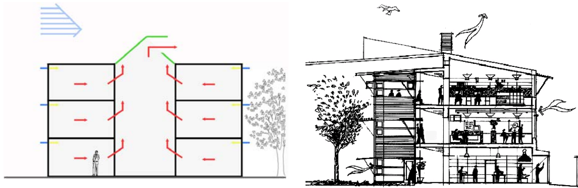
Figure 3. The concept of façade ventilation. The right figure shows Prestetrød school (source: White Arkitekter AB).
