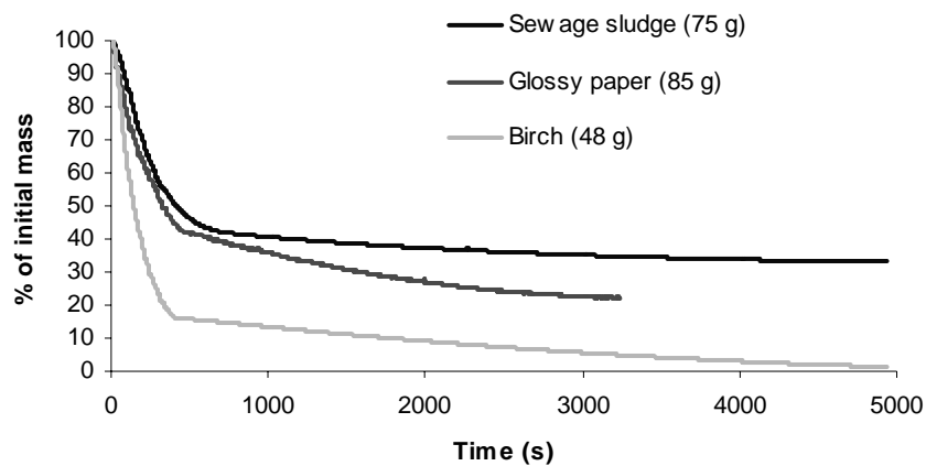
Fig. 6 Mass loss curves for the three fuels at 750°C (initial reactor temperature, the corresponding temperature profiles are shown in Figure 4).
