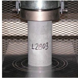
(a) Cylinder compressive test.
