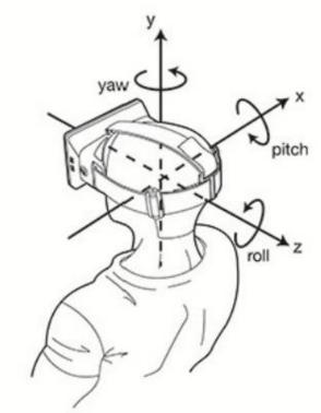
Figure 2: Orientation Directions (20)
