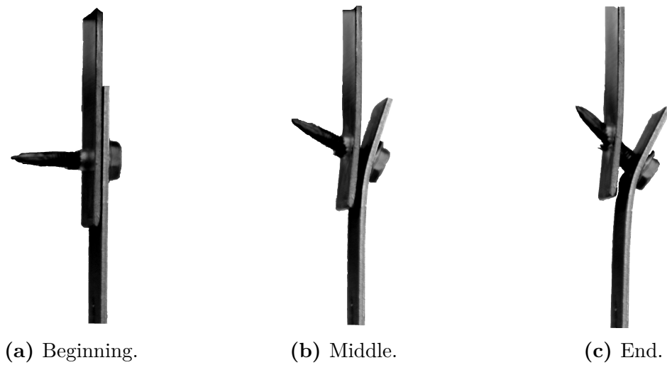
Figure 4.11: Deformation progress for the lap-joint.
