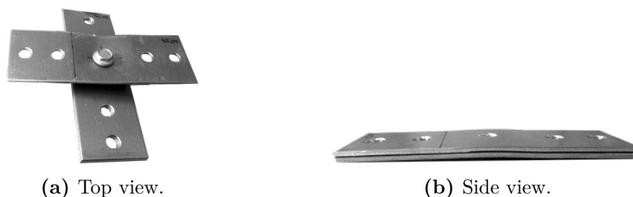
Figure 4.26: Deformation of cross type 3 specimen under mixed loading.
