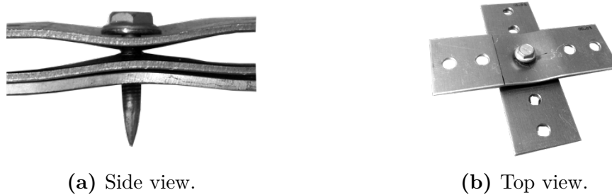
Figure 4.24: Deformation of cross type 3 specimen under tensile loading.
