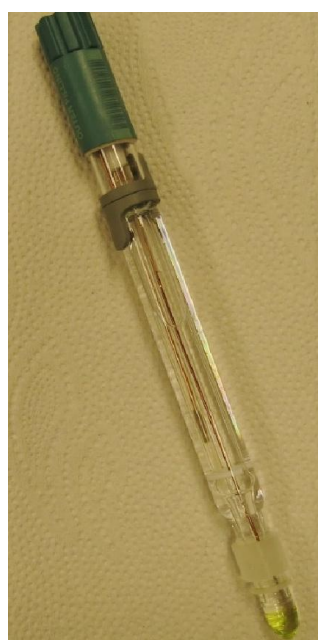
Figure 3.4 - Metrohm Profitrode used for pH measurements
