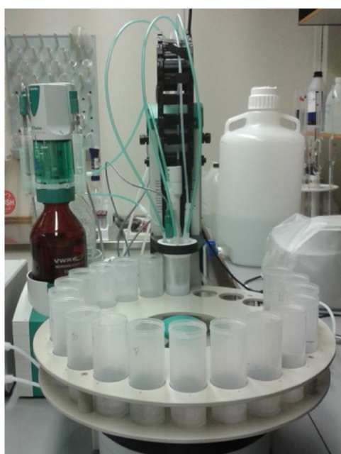
Figure 3.3 - Automatic potentiometric titration from Metrohm
