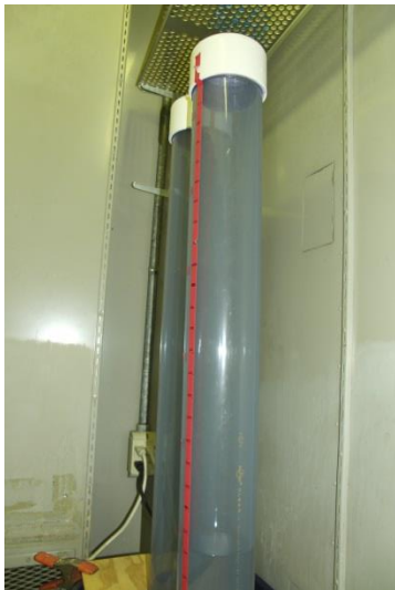
Figure 4 - Columns used for gas volume measurements. Based on water displacement.
