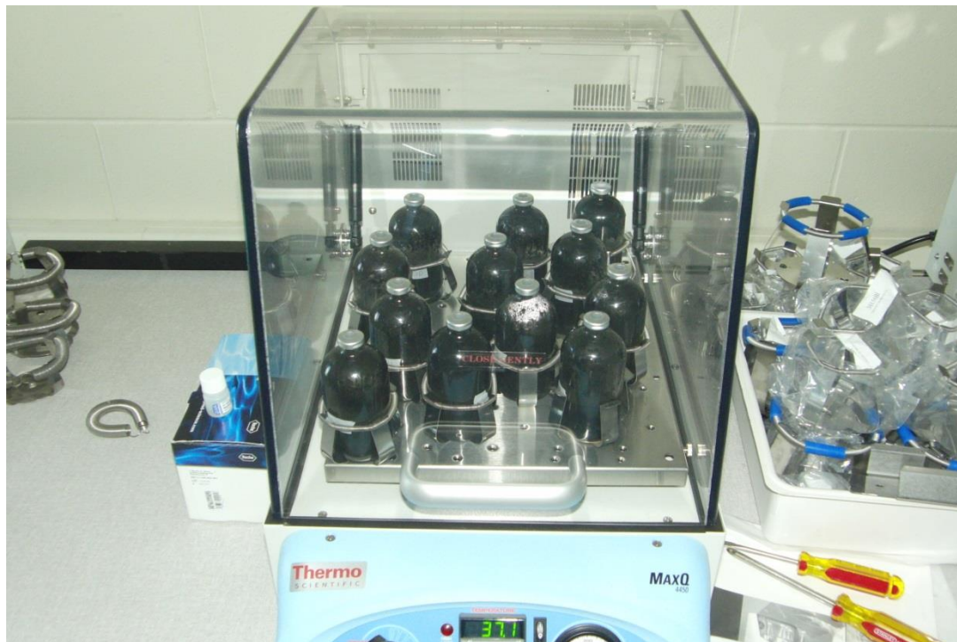
Figure 13 - Shaker table at which the reactors were put. The temperature is set to 37° C; the table is set to 80 rpm.
