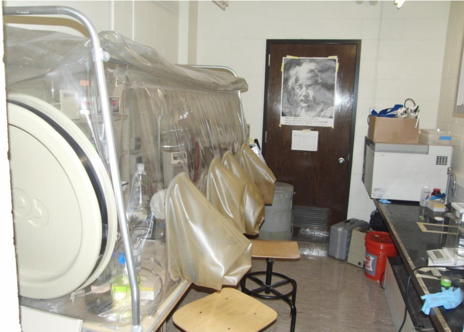
Figure 12 - Glove box used in the feeding and spiking of the reactors. Makes it possible to work in an oxygen free environment.
