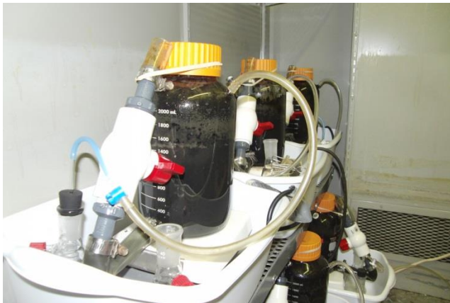
Figure 3 - Bench-scale reactor with sludge volume of 1.5 L
