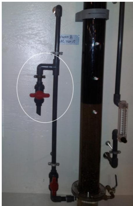
Figure 15: Sample port at the filter column effluent (marked with a white ring)
