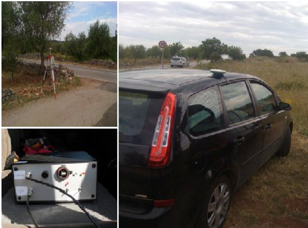
Fig. 3.2a (on the upper left): Master antenna above the survey point. Fig. 3.2b (on the right): Rover antenna on the car top. Fig. 3.2c (on the lower left): Rover receiver inside the car
