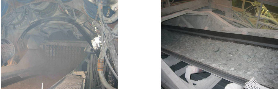
Figure 4. Dust & transport differences: left side water use, right side MEYCO ABR 5.
