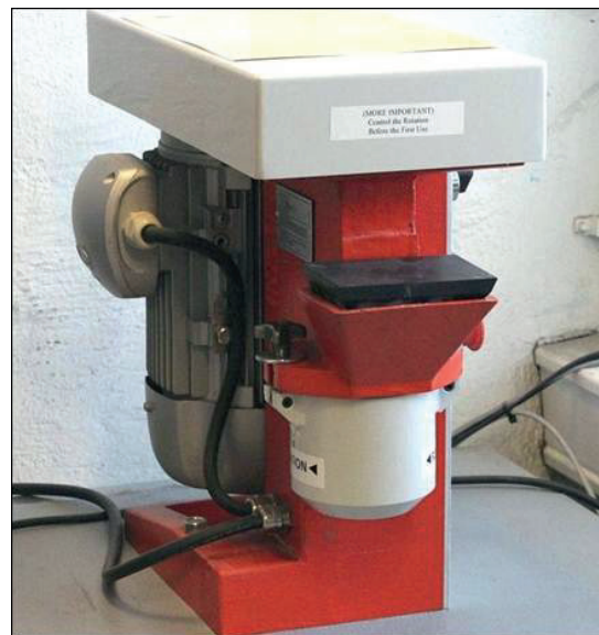
Figure 3: The LCPC test apparatus (Photo by Filip Dahl).
