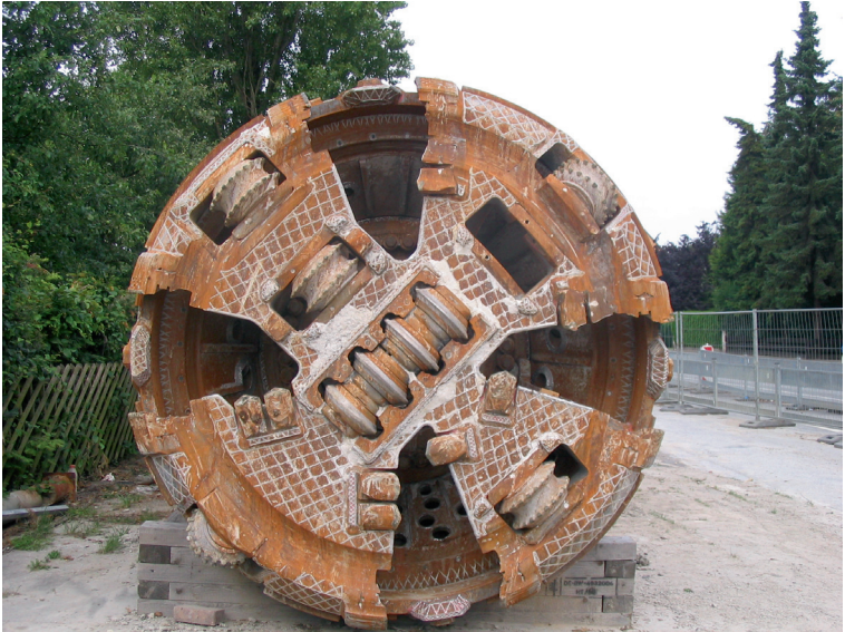
Figure 9 Damaged cutter head after the second drive at the Sammler Ost project. (Photo: Tim E. E. Becker)
