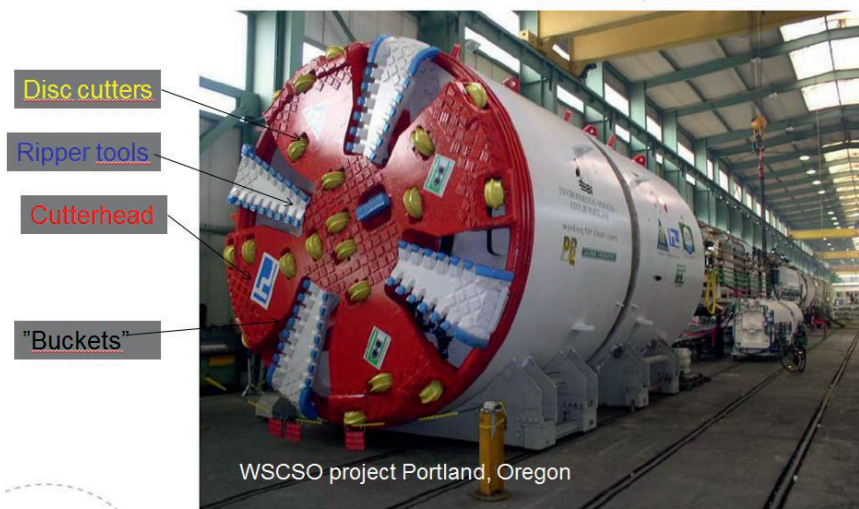
Figure 6. Mixed condition cutter head fitted with scraper/ripper tools and disc cutters. Photo; Herrenknecht.
