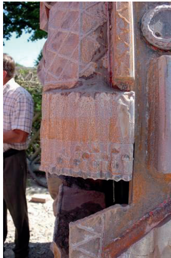
Figure 5. Worn-out carbide inserts and hard facing on a scraper/reamer tool due to abrasive wear. Photo by Tim E. E. Becker.
