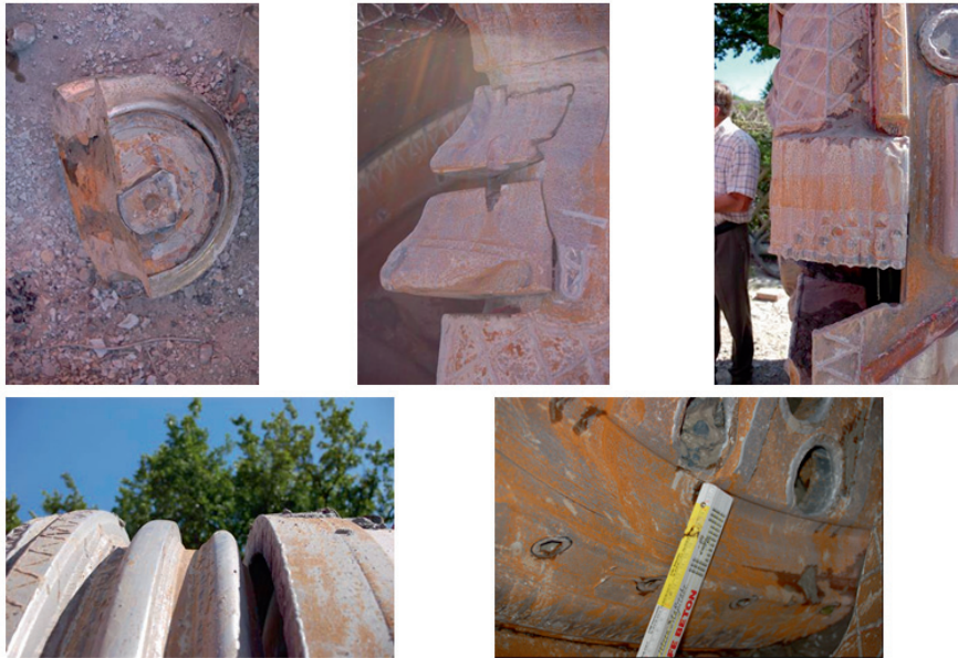
Figure 10 Photo showing blocked and destroyed double disc cutter (up left), worn out ripper tools (up middle), worn out scraper tools (up right), reduced cutter head diameter (down left) and worn out front of cone crusher (down right). (Photos: Tim E. E. Becker)
