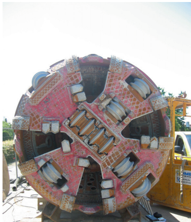
Figure 7 Photo of the cutter head of the Herrenknecht pipe jacking machine AVN 1600/1800. (Photo: Tim E. E. Becker)
