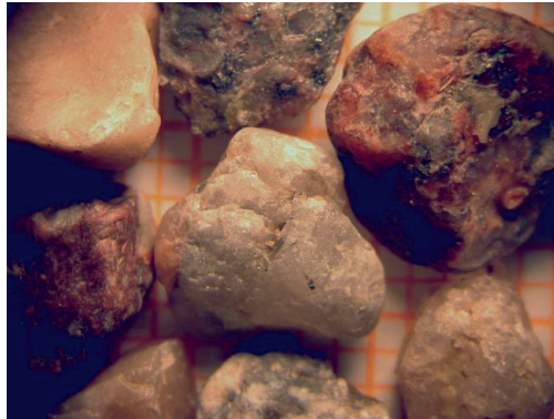
Figure 11 Photo of typical grain shape of the sand and silt sections in the analyzed project (orange grid is 1/10 mm)
