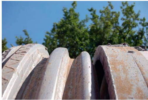
Figure 4. Reduced cutter head diameter due to abrasive wear to hard facing. Photo by Tim E. E. Becker.
