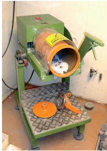
Figure 14. The Ball Mill Test apparatus can be used to assess the reduction in abrasivity resulting from introducing water and/or soil conditioning additives. The test apparatus consists of a rotating drum filled with soil (0 - 16 mm diameter) and 20 steel bits.
