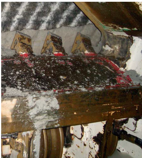
Figure 2: Double disc cutter and scraper tools in contact with a mixed face consisting of claystone and gypsum (Photo by Pål Drevland Jakobsen)
