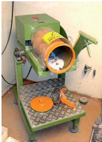
Figure 9: Ball Mill Test apparatus can be used to show the reduction of abrasivity by introducing foams.
