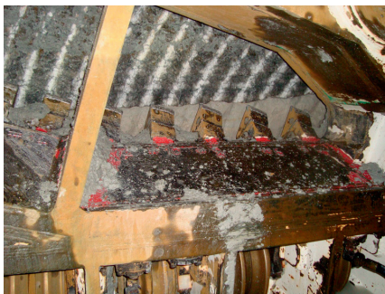
Fig. 2. Double disc cutter and scraper tools in contact with a mixed face consisting of claystone and gypsum. The simplified laboratory approaches presented in this paper cannot fully recreate the complex tribological system shown in the photo. Such approaches enable researchers to assess different soil grains abrasivity and impact on TBM tools separately (Photo by Pål Drevland Jakobsen).
