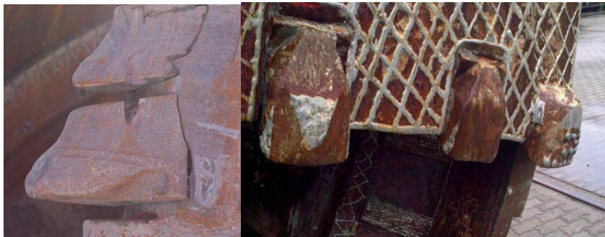
Figure 3. Worn-out ripper tools abrasive wear. Photo by Tim E. E. Becker.
