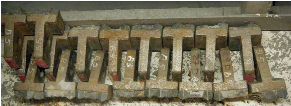
Figure 60. Worn-out scraper tools from slurry TBM used for assessment of the validity of the estimators in the PhD study (Photo by Wojtek Smolen).
