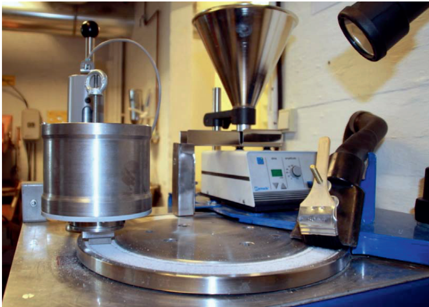
Figure 5. The NTNU/SINTEF Abrasion Test apparatus.
