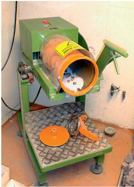
Fig. 9. Ball Mill Test apparatus can be used to assess the reduction of abrasivity by introducing soil conditioning additives. The test apparatus consists of a rotating drum filled with soil (0–16 mm) and 20 steel bits. Water and/or soil conditioning additives can be applied.
