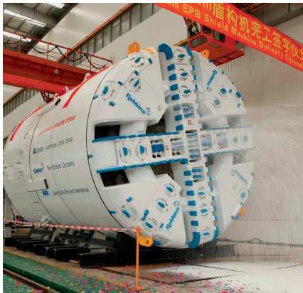
Fig. 1. Earth Pressure Balance shield (EPB) TBM with foam nozzles (Courtesy by the Robbins TBM Company).
