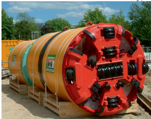
Figure 2 Newly manufactured pipe jacking machine, AVN 1600/1800 TB by Herrenknecht. (Photo: Tim E. E. Becker)
