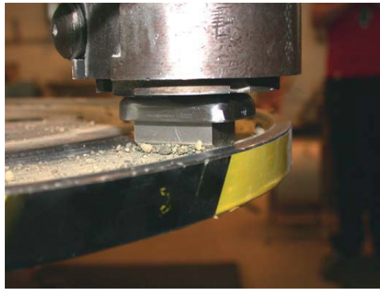
Figure 33. Interaction between dry and loose soil particles and the steel bit during an SAT TM test (Photo by Filip Dahl).
