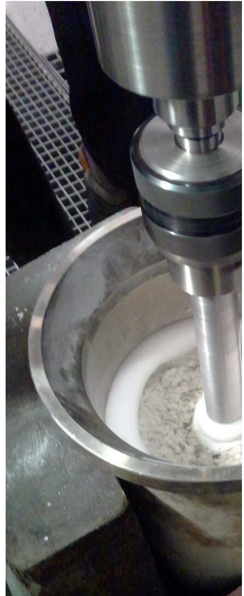
Left, top: Figure 3, hyperbaric test chamber 150 x 300 mm; Above: Figure 4, boring in to a compacted soil sample with soil conditioning foam under atmospheric test conditions
