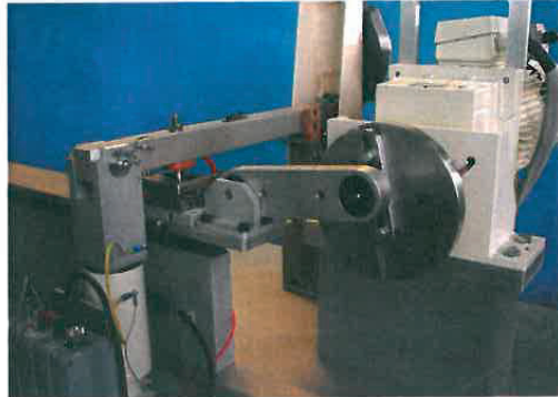
Above: Measuring wear and contact behaviour
