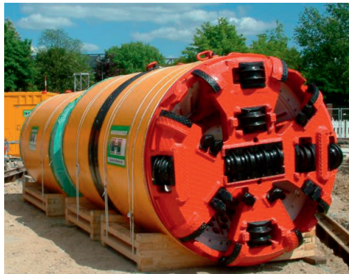
Figure 2 Newly manufactured pipe jacking machine, AVN 1600/1800 TB by Herrenknecht AG. (Photo: Tim E. E. Becker)
