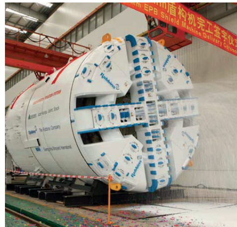
Figure 1: EPB TBM with foam nozzles (Photo by Robbins TBM Company)
