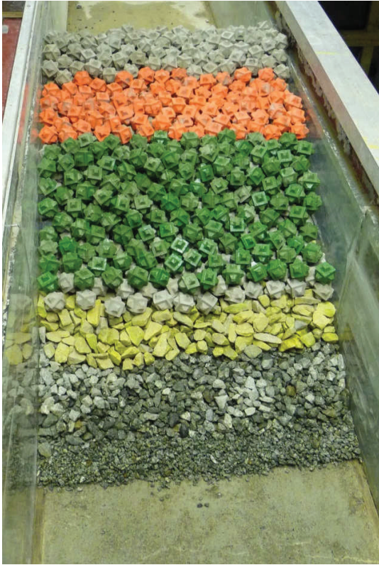
Figure 37. Breakwater before any wave step
