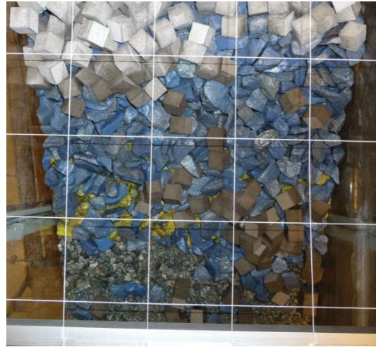
Figure 11. Breakwater front after step 5
