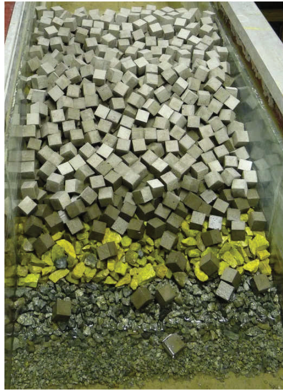
Figure 16. Breakwater after wave step one
