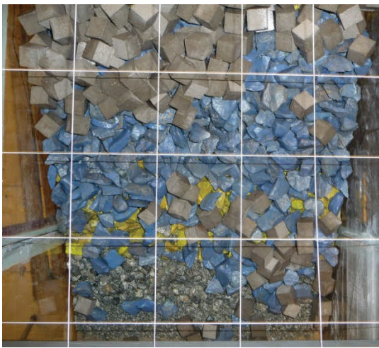
Figure 10. Breakwater front after step 4
