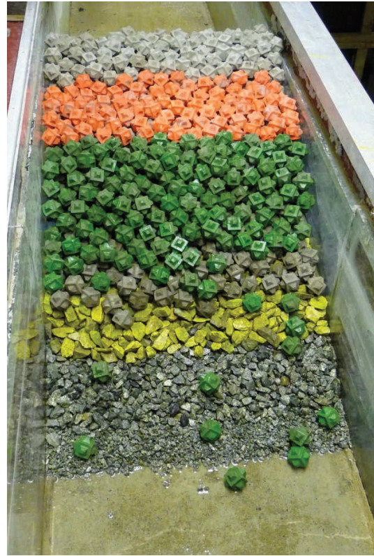
Figure 38. Breakwater after wave step one
