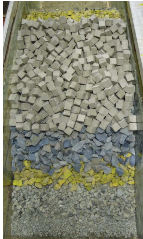
Figure 6. Second layer concrete cubes
