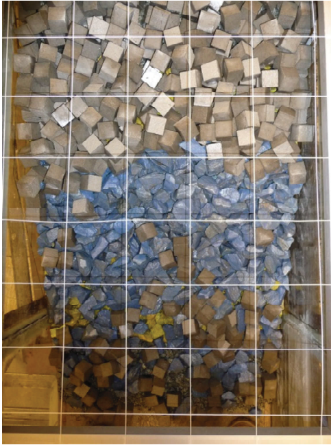
Figure 12. Breakwater front after step
