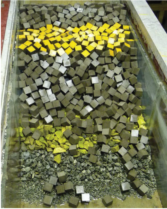
Figure 30. Breakwater after wave step four
