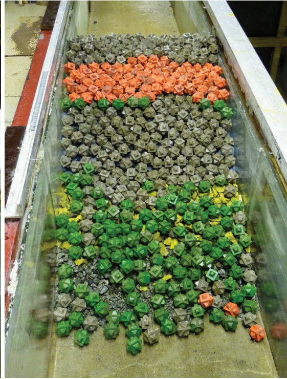
Figure 53. Breakwater after wave step five
