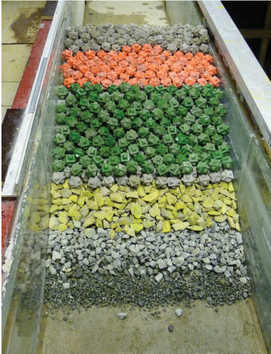
Figure 48. Breakwater before any wave step
