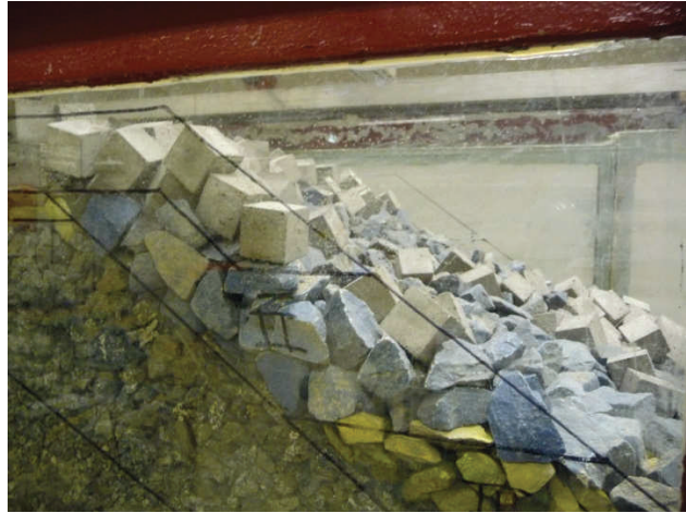
Figure 13. Breakwater profile after step 6
