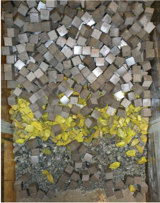
Figure 19. Breakwater after wave step four
