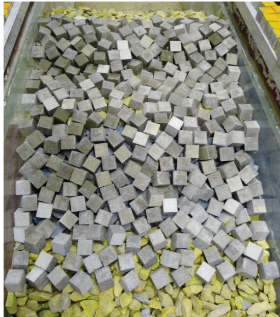
Figure 23. First layer of concrete cubes
