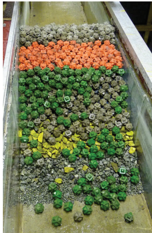
Figure 40. Breakwater after wave step three
