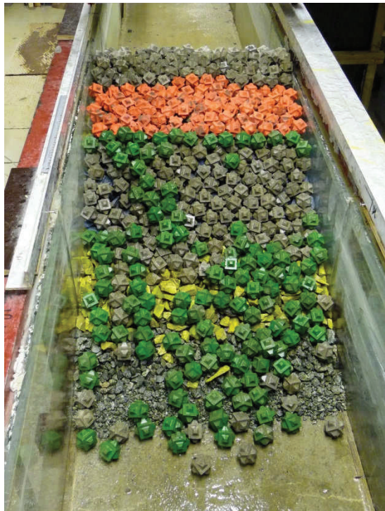
Figure 51. Breakwater after wave step three
