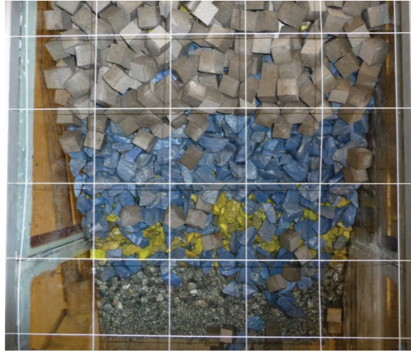
Figure 9. Breakwater front after step 3
