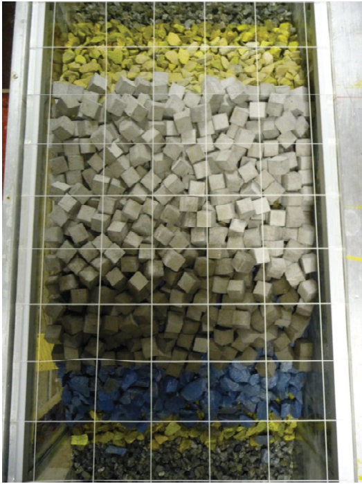
Figure 8. Breakwater after running wave step one
