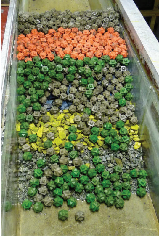
Figure 41. Breakwater after wave step four
