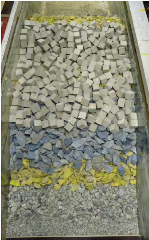
Figure 5. First layer concrete cubes
