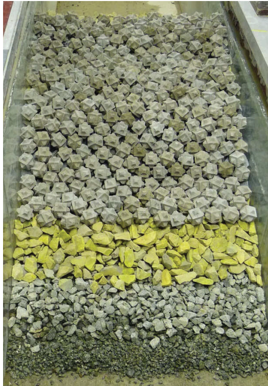
Figure 45. First layer of cubipods
