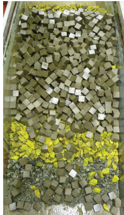
Figure 18. Breakwater after wave step three
