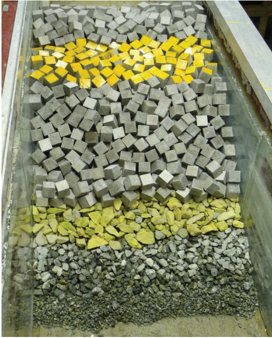
Figure 26. Breakwater before any wave step
