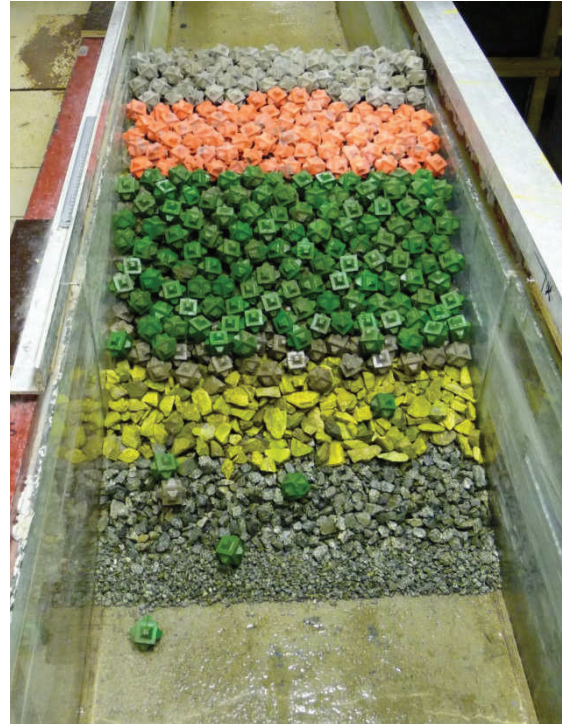
Figure 49. Breakwater after wave step one
