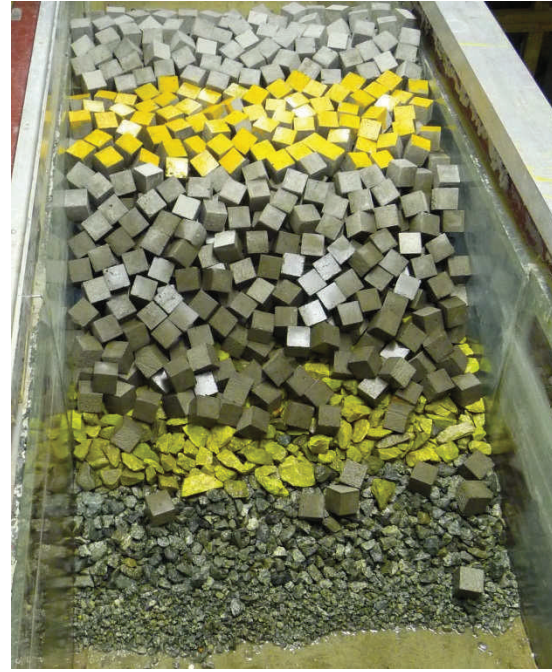
Figure 27. Breakwater after wave step one
