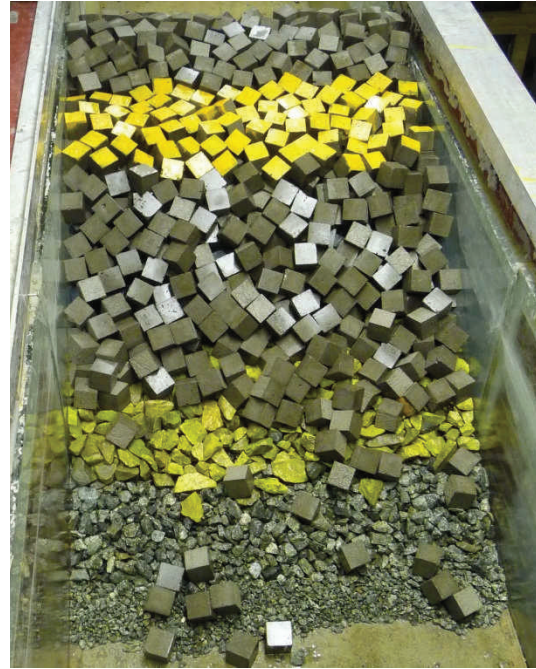
Figure 29. Breakwater after wave step three
