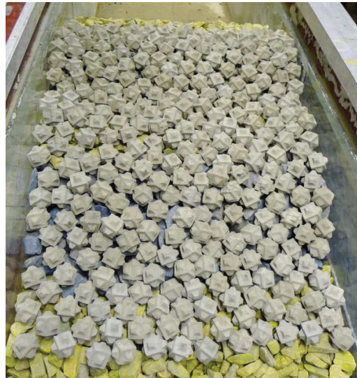
Figure 34. First layer of cubipods
