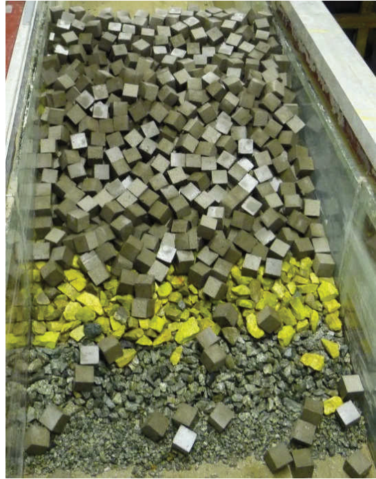
Figure 20. Breakwater after wave step five
