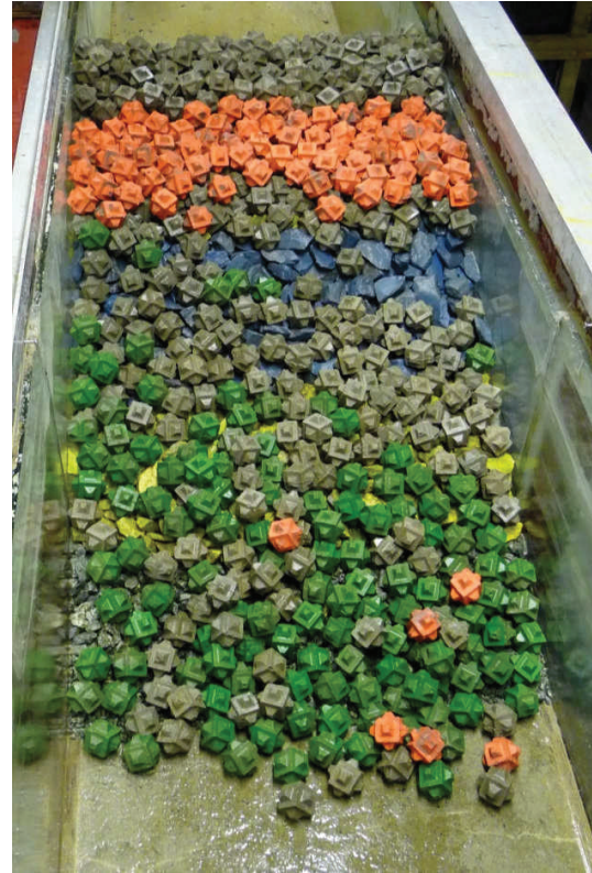
Figure 42. Breakwater after wave step five
