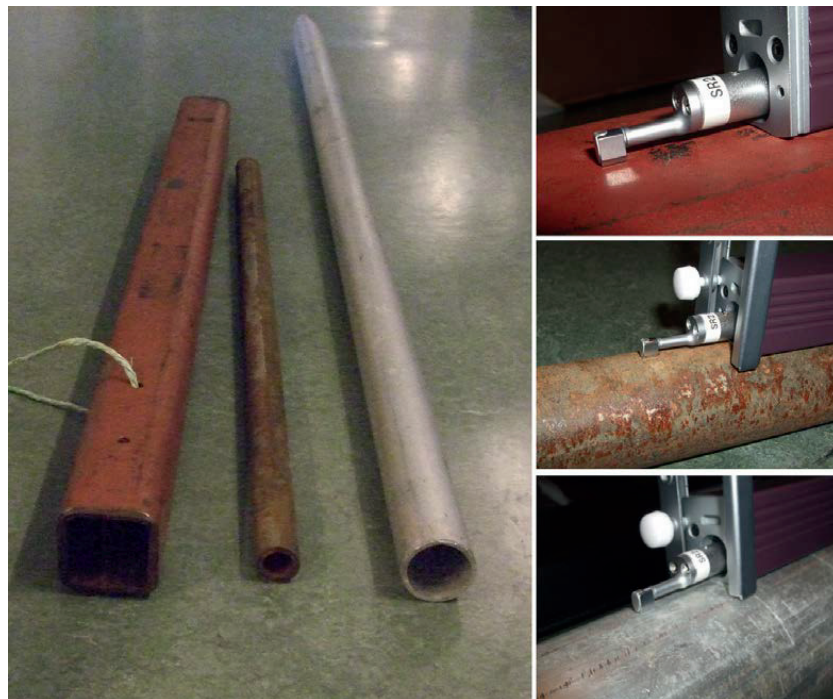
Figure 5.4. Ice piles used in the tests (left photo) and measurements of their roughness.
