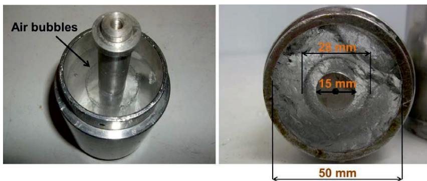
Figure 4.9. Ice formation in the annulus between the hollow cylinder and a coaxially located steel piston.
