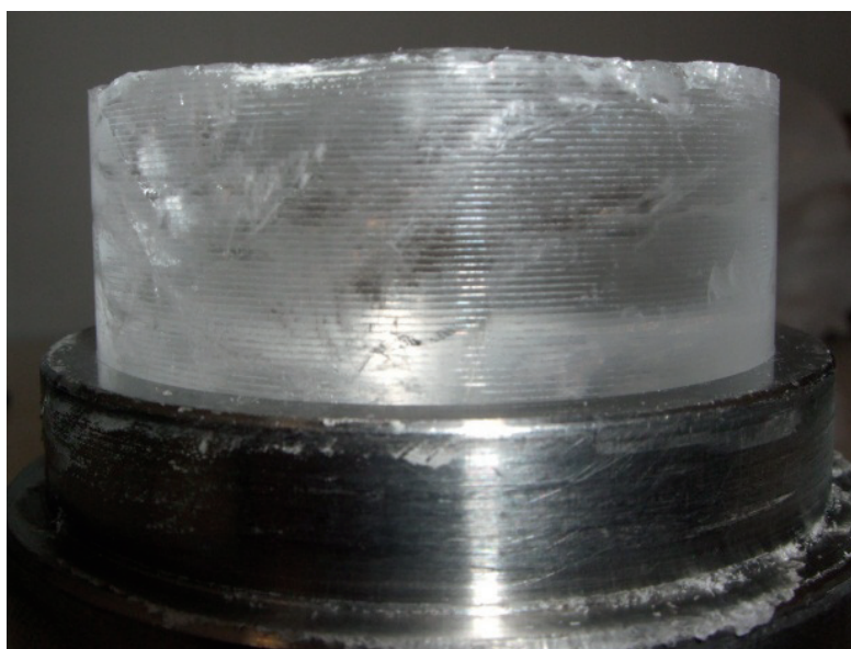
Figure 4.13. Ice surface after testing of sample Mr filled with freshwater ice.
