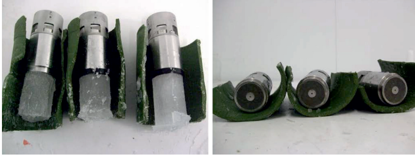
Figure 4.10. Samples containing salty ice after their extraction from the ice tank (left) and after the sawing process (right).
