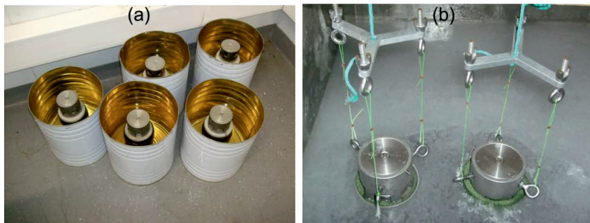
Figure 4.8. (a) Freshwater ice and (b) salty ice formation in the annulus between the piston and ice.
