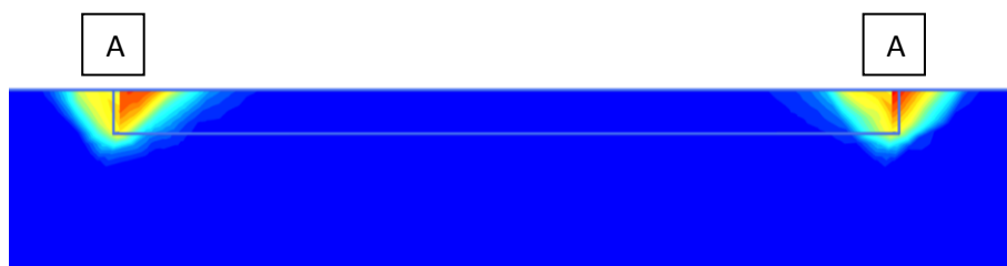
Figure 5.8: Total displacement under H_{ult} illustrated with shadings of A-A cross section
