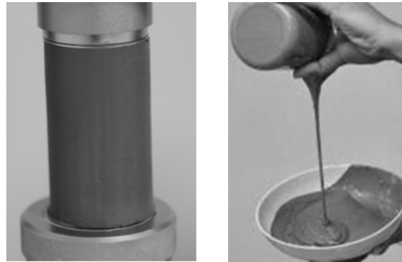
Figure 2 :A highly sensitive clay in the intact (left) and fully remolded states (right).
