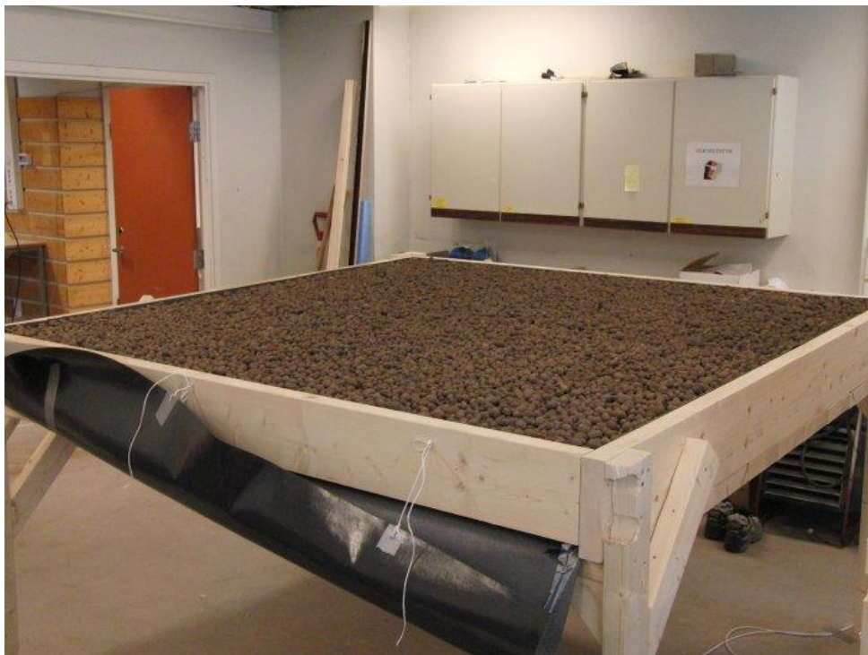
Figure 19. One of the two wooden crates filled with Leca ® 10-20mmR.
