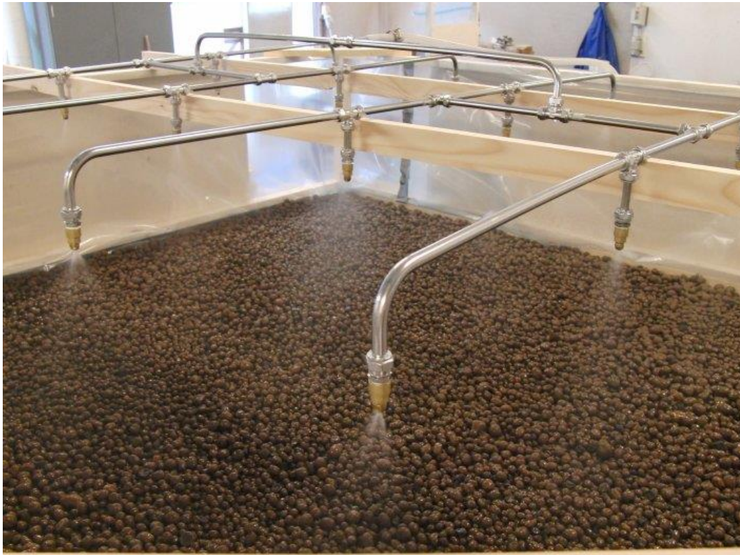
Figure 20. The nozzles spreading water, simulating rain, over Leca® 10-20mmR.
