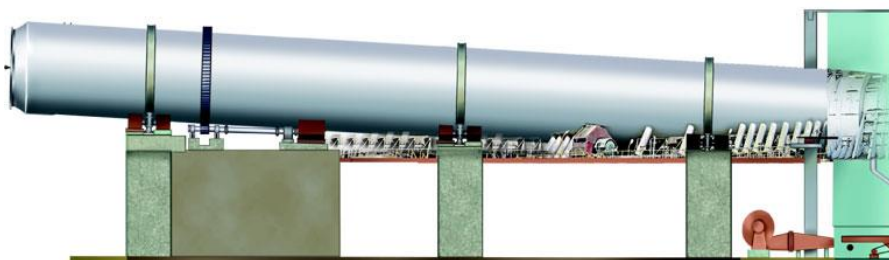
Figure 10. Rotary kiln the length is usually between 30 to 60 meters depending on the composition of the raw material the different producers are using. [12]
