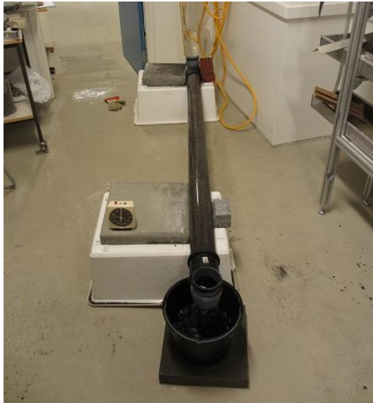
Figure 27. A test of the permeability being performed.
