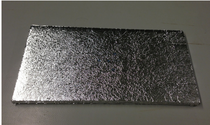
Fig.4 VIP panel Vacupor NT-B''-S from Porextherm, used in this study
