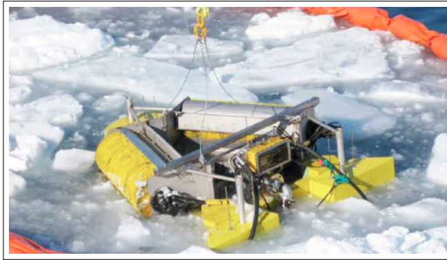
Figure 8.4: Skimmer prototype "Framo" during field testing in the Barents Sea in 2009. Source: SINTEF
