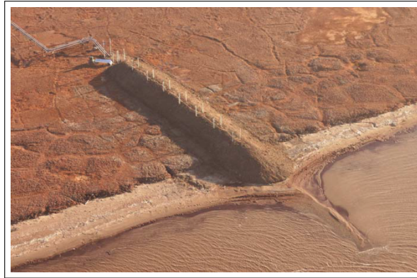
Figure 9.7: Oooguruk shore crossing aerial photograph. Source: G. Lanan et al., 2008
