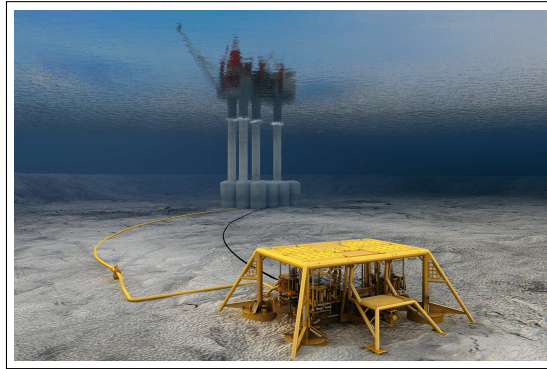
Figure 4.6: Subsea template with four wells tied to the fixed platform at Gullfaks C in the Norwegian North Sea. Source: Statoil
