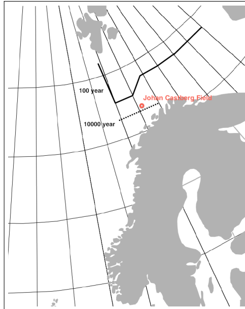
Figure 11.5: Limit for collision with icebergs at the field location. Source: Modified from NORSOK N-003
