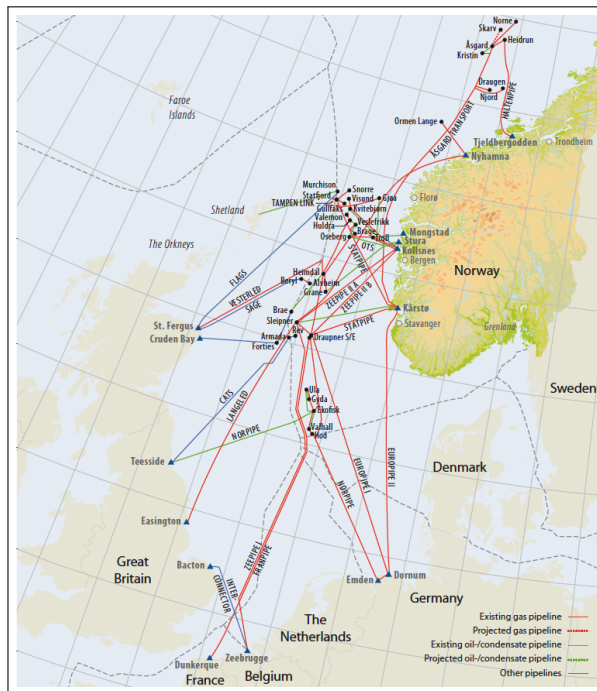
Figure 5.6: Existing and projected pipelines on the Norwegian Continental Shelf. Source: The Norwegian Petroleum Directorate
