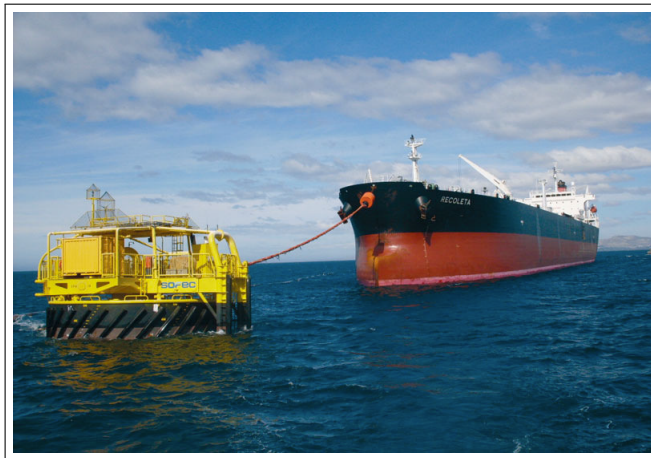
Figure 6.3: Single buoy mooring. Source: BMT Scientific Marine Services
