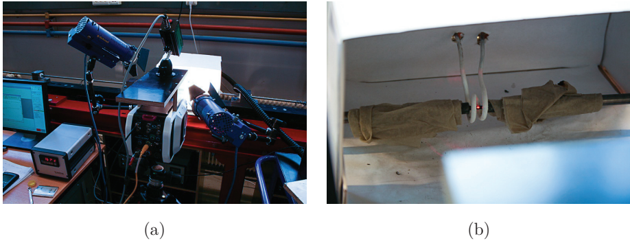
Figure 3.7: (a) Overview of test setup where two light sources, the pyrometer and the high-speed camera can be seen and (b) test specimen mounted in test rig together with coil and laser beam
