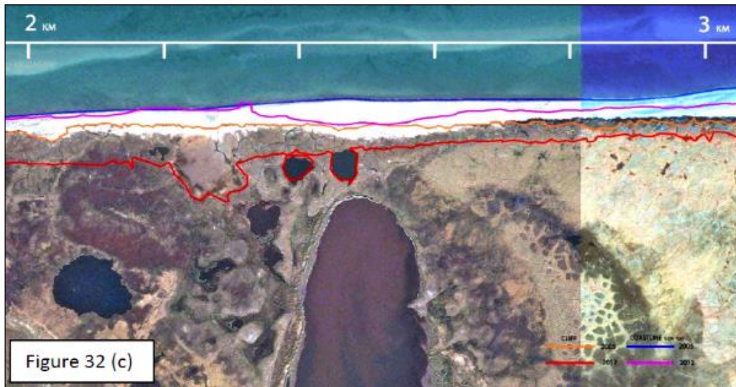
FIGURE 4.5 API AND GIS MAPPING - POSITION OF COASTLINE AND CLIFF LINE OVER 7 YEARS (SOURCE: SAMCoT REPORT, 2013)
