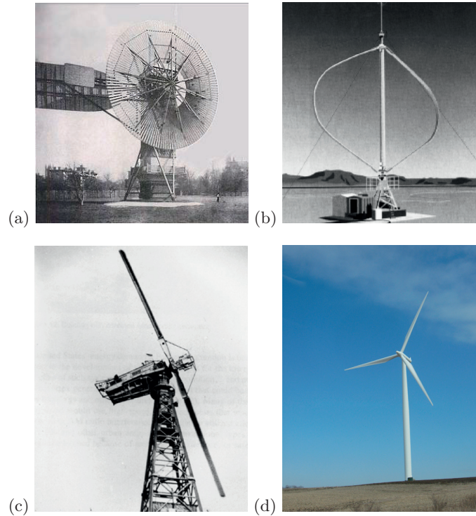
Figure 1.1: Different wind turbine concepts; (a) worlds' first automatically operated wind turbine, courtesy to [1], (b) Darrieus vertical axis wind turbine, courtesy to [2], (c) worlds first MW size wind turbine, courtesy to [2], and (d) today's conventional three bladed horizontal axis wind turbine.
