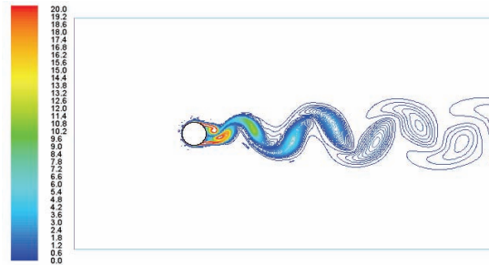
Fig 5: Vortex shedding behind the monopile. Colors represent vorticity magnitude.
