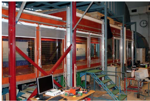
Figure 1 Wind tunnel at NTNU's aerodynamic laboratory, length 11 m, height 1.9 m and width 2.7 m.
