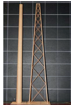
Figure 2 Tubular and truss tower (left and right, respectively) used in the wind tunnel experiment.
