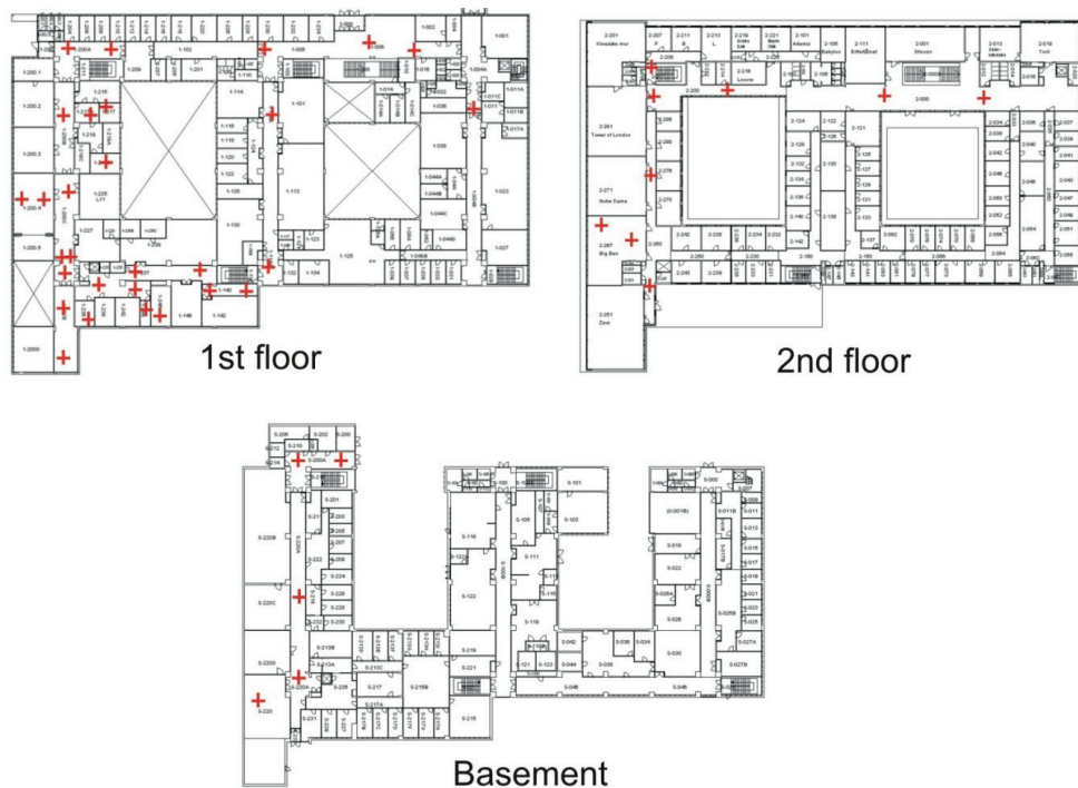
Figure 2: Control points established in the building.
