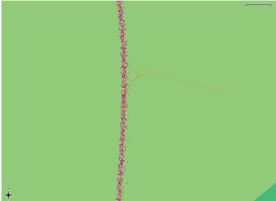
FIGURE 52 PLOT OF GPS DATA ALONG THE E6 AT HJERKIN (OPEN MOUNTAIN SURROUNDINGS)
