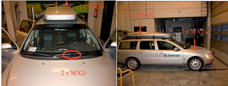
FIGURE 54 PLACEMENT OF GPS LOGGERS IN TEST VEHICLE
