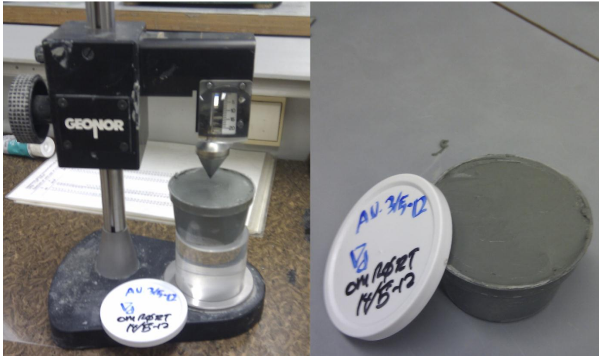
Figure 19 Remolded sample stored in plastic cup prepared for thixotropy fall cone test
