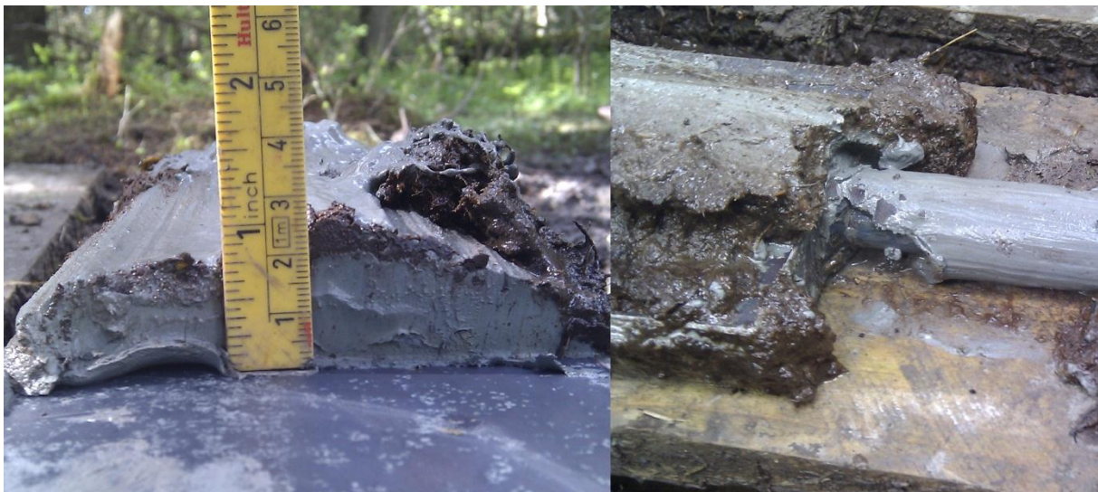
Figure 54 Deep-seated clay on steel plate (left hand side) and clay behavior in the transition zone from plate to rod (right hand side)
