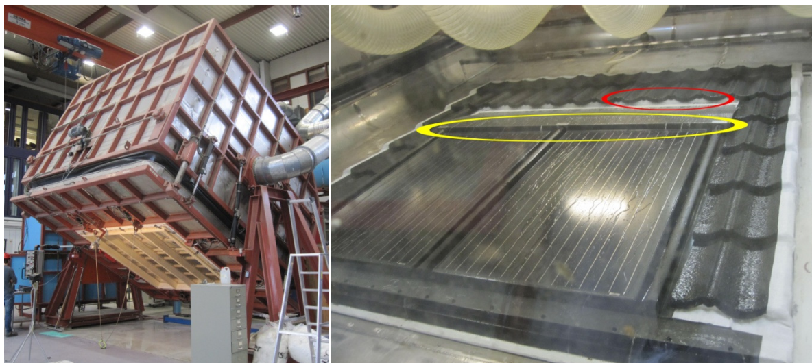
Fig. 5: Visual inspection of BIPV sample roof from below the inclined RAWI box (left) and sample roof inside the RAWI box during testing, viewed from outside the box through a window (right). The coloured ellipses denote leakage points.
