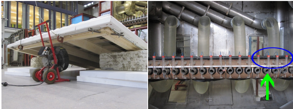
Fig. 6: Drying of BIPV sample roof with fan heater between test phases (left), and the boom inside the RAWI box which delivers wind-driven rain across the sample area (right). Water runs from the blue tubes on top (blue ellipse), drips down the transparent vertical cylinders (blue ellipse), and is blown onto the sample area as it hits the air stream that blows out of the air tubes (green arrow).
