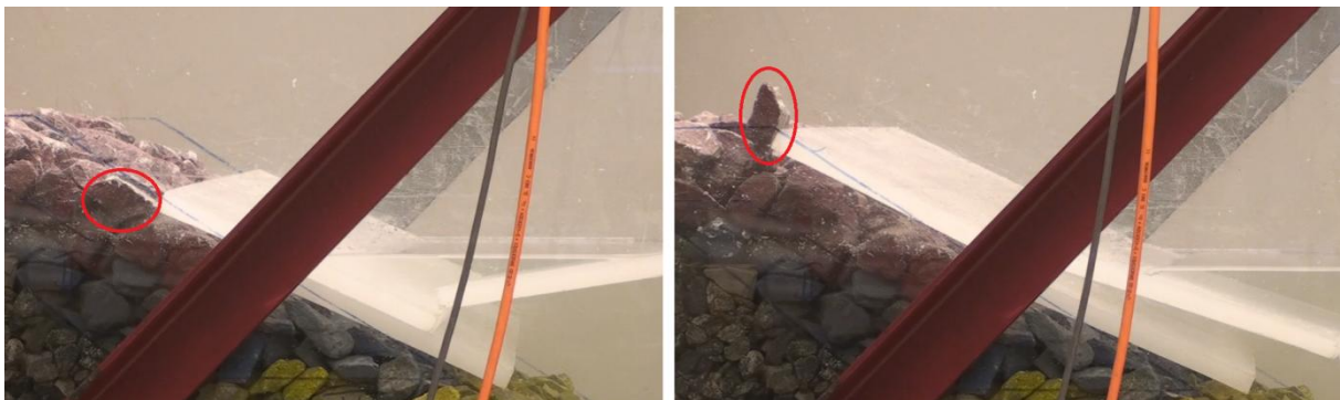
Figure 32- Test 59 (TESTS1FF): motion of an individual stone
