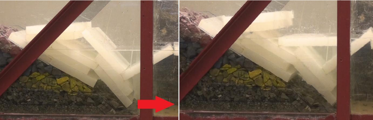
Figure 28- test 15(TESTS1E): Accumulation in front of the breakwater scrapping the toe of the breakwater. The red arrow shows the movement of the model ice
