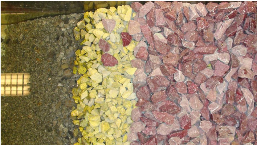
Figure 26-Test 3bis(TESTS1D): stones from the top of the breakwater have been dragged downward the rear slope
