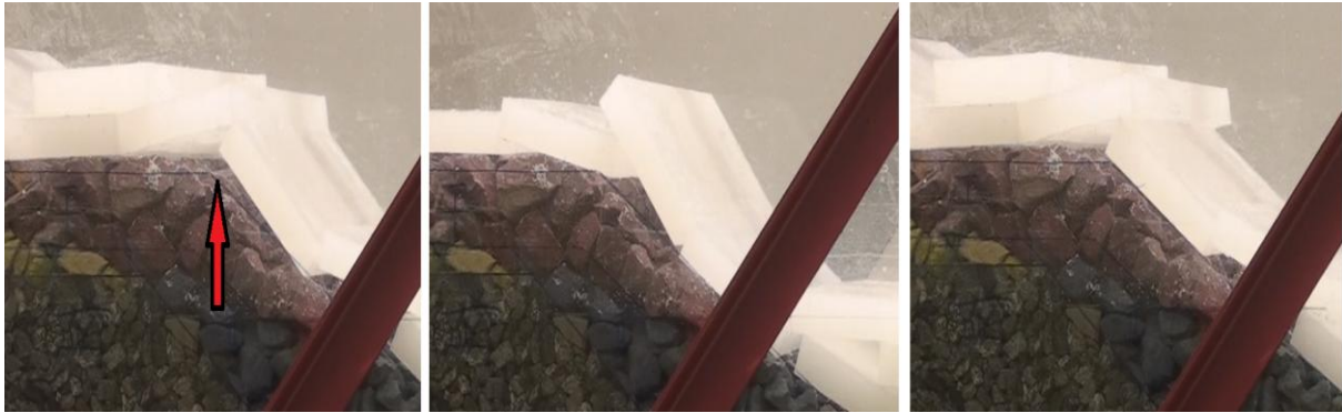
Figure 16-from left to right: upward force lifting the plates; incoming plate sliding on top; incoming plate sliding below.
