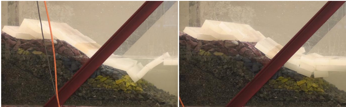
Figure 17-Possible accretion after ride up. On the left, the test 18 at the moment of the release ( about 800s). On the right the same test some minutes after the release
