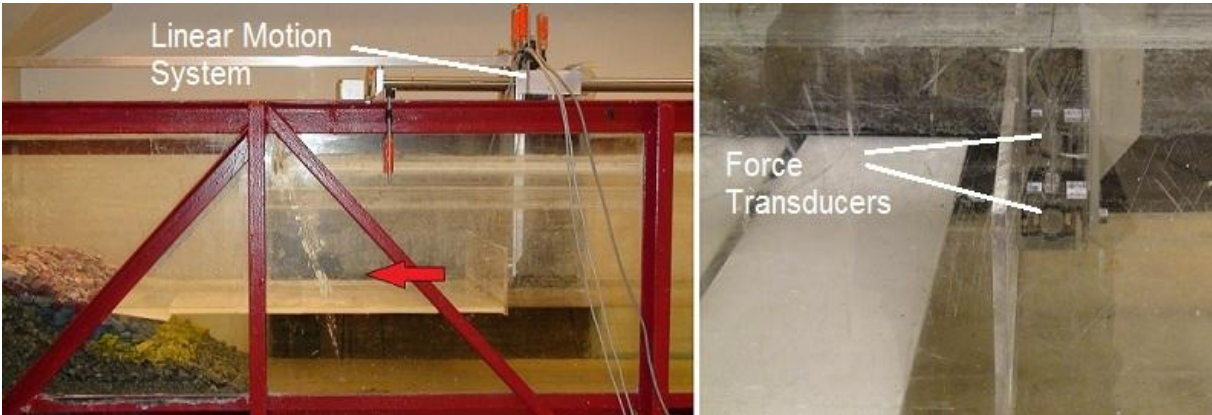
Figure 11-Linear motion system and force transducers
