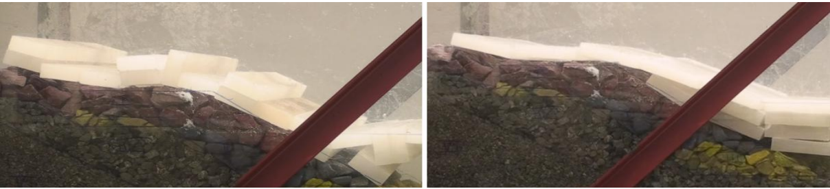
Figure 27-Test34(TESTS1FA) on the left and test39(TESTS1FC) on the right. Most advanced ride up events during tests with added friction.
