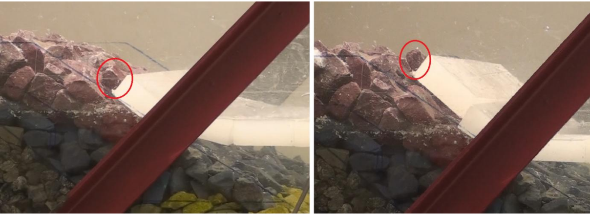
Figure 25-Test 17(TESTS1A): a stone is moved up the slope
