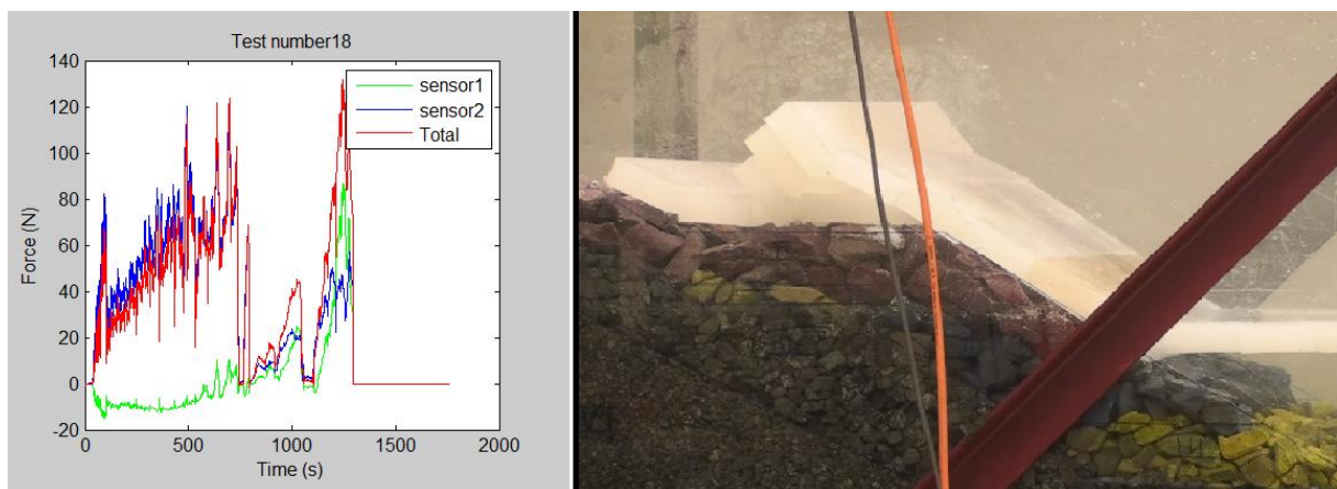
Figure 15-Test18(TESTS1A): Typical ride up phenomenon
