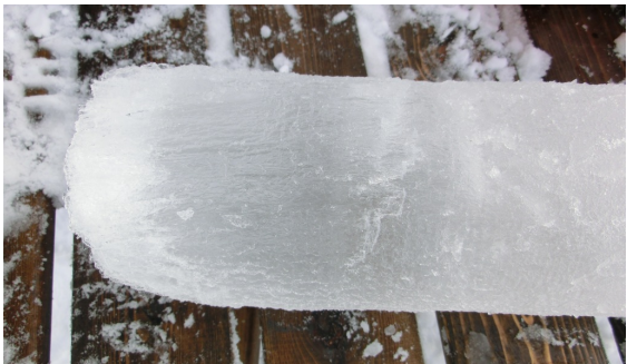
Figure 35: Close-up of the skeleton layer. Brine pockets are present in the core.
