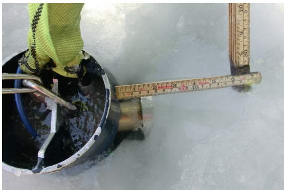
Figure 60: An attempt of measuring the displacement of the indenter at BH E3.2.
