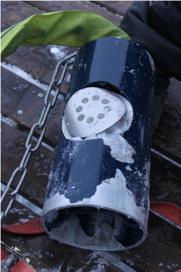
Figure 36: The indenter twisted about 45° in Test 5, A1.5.
