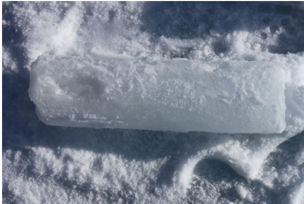
Figure 87: Bottom 30 cm of H3 extracted as one core. Large brine pocket (left) located at 105 cm depth.
