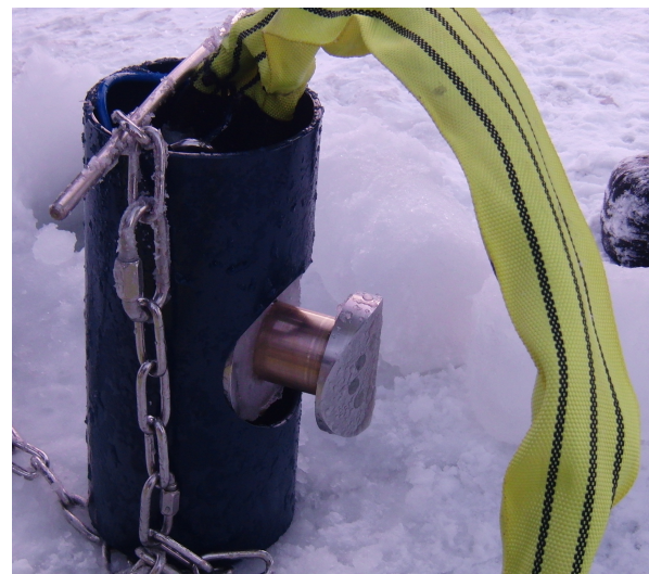
Figure 8: The jack with piston fully extracted, 50 mm.
