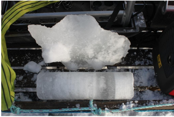
Figure 68: Core and Fragment C from spalling failure in Test 12 (C3.4).
