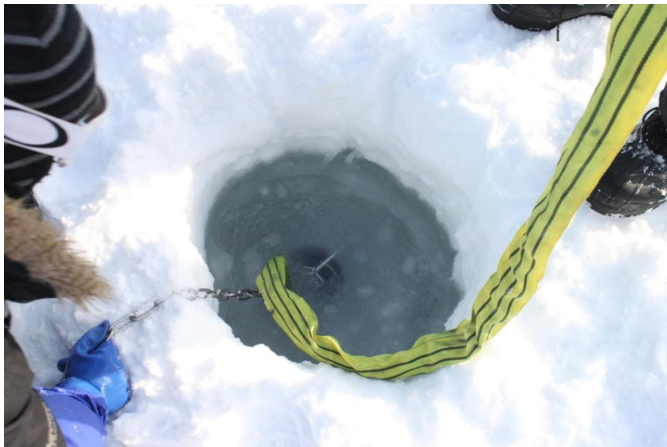
Figure 47: Slush preventing the BHJ crew from observing the failure (if any) in the ice surface of an arbitrary test.
