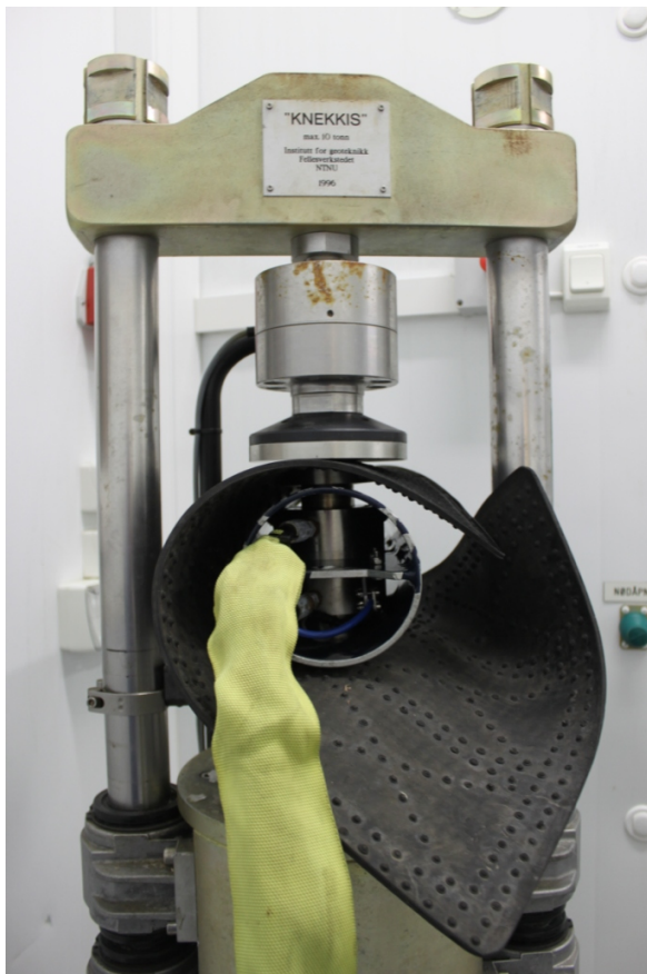
Figure 15: The jack with a rubber mat placed in the jaws of Knekkis during calibration.
