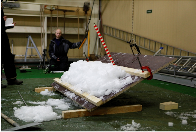
Figure 23: Tilting of pile test 2060
