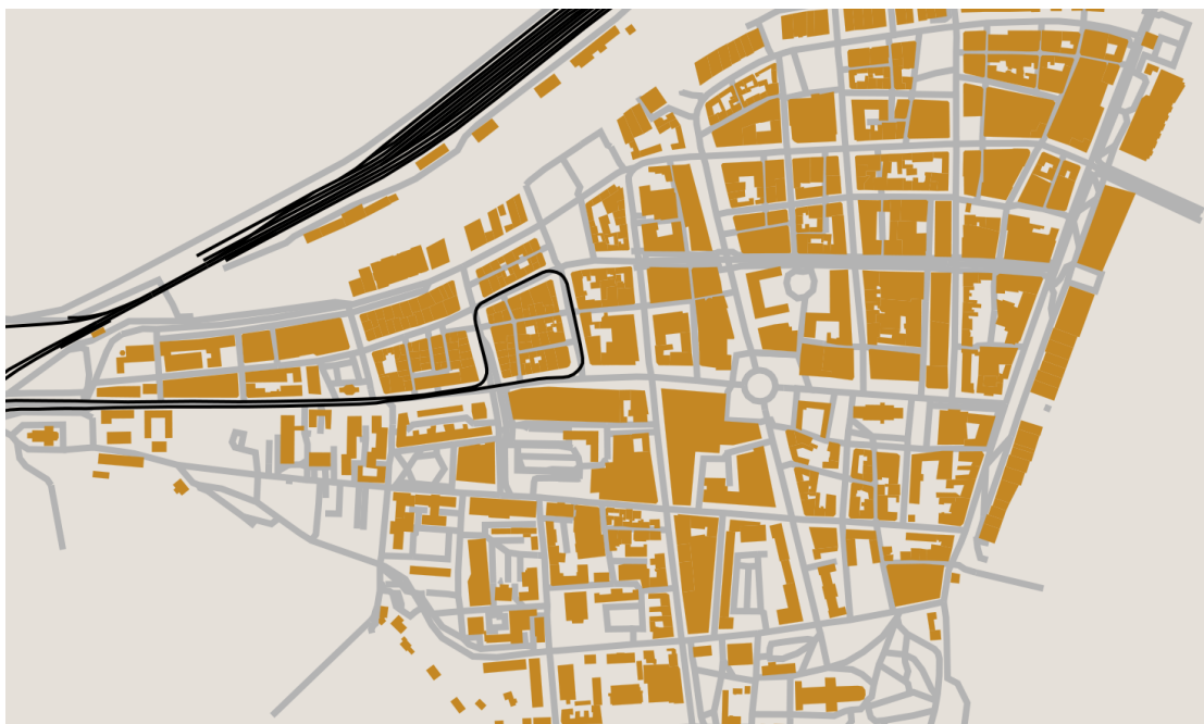
Figure 5.7: Illustration of a pure vector tile application. Seen here is an area from the centre of town in Trondheim, with roads, buildings and railway lines drawn on the map.
