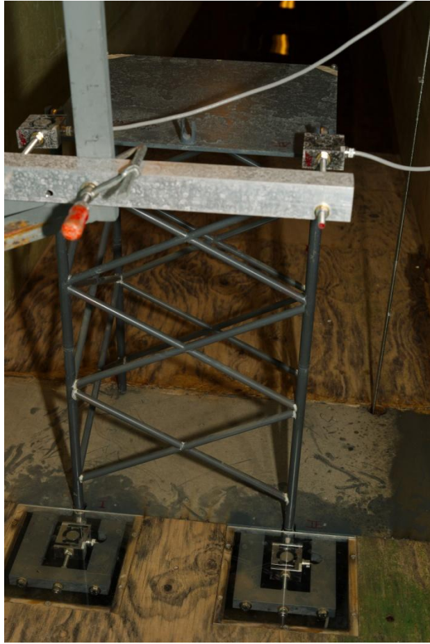
Figure 28: Structure with force transducers
