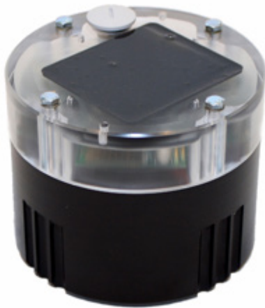
Figur 14 STMS magnetometer (Sensebit, 2011)
