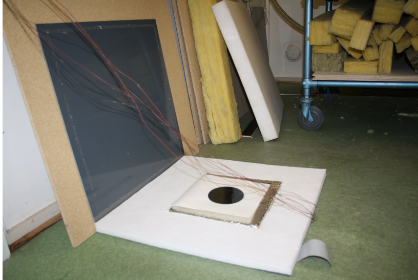
Figure A2. The customised setup for smaller test pieces. The heat flow meter is the black, circular plate in the middle of the frame.
