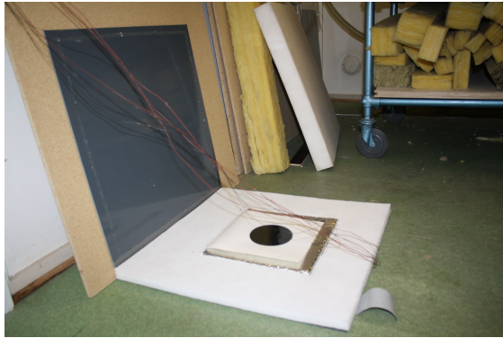
Figure 3. The customized setup for smaller test pieces, used in the heat flow meter.
