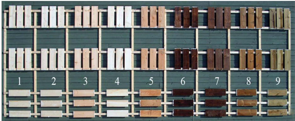
Figure 5.1.: Photo of the test setup at the Voll test site, Trondheim. West facing wall, February 2005, numbers refer to material numbers from Table 5.1.
