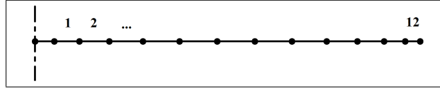
Figure B.3: The distribution of elements (both structural and aerodynamic) along the blade
