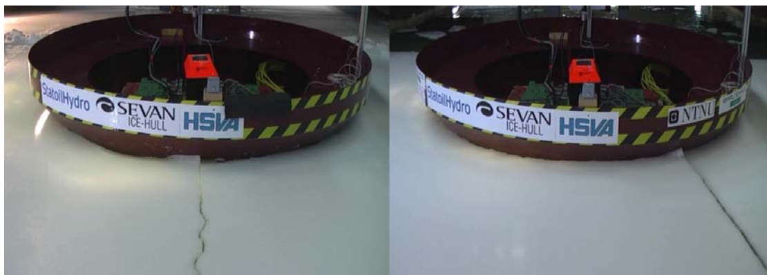
Figure 3.8 The observed huge radial cracks in Test #3130 (left) and #4110 (right)
