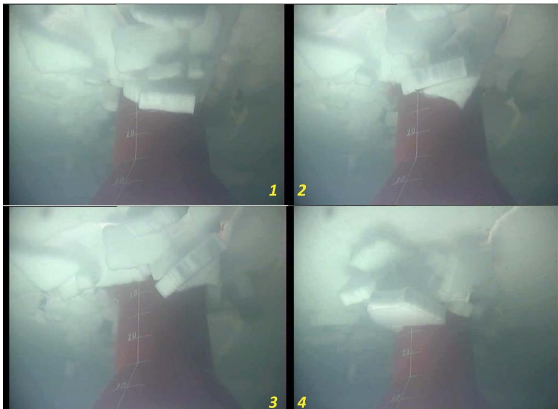
Figure A. 7 Loading process of Model B_F in managed ice (large floes)
