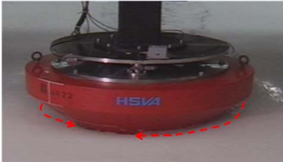
Figure 4.3. The water flush-in with indication of direction and area above the broken ice for an ice speed of 0.5 m/s. (The photo was visually cut from the video just before the next breaking and the water flush-in area was processed visually as well; the area above the broken ice is partially ventilated).
