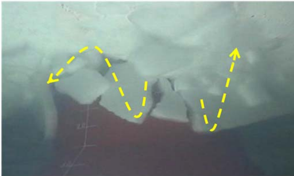
Figure 4.25. Photo of Model D_F's ice clearing ability in managed ice. (30 m×50 m managed ice; in Test #02Li42; ice speed 1 m/s).
