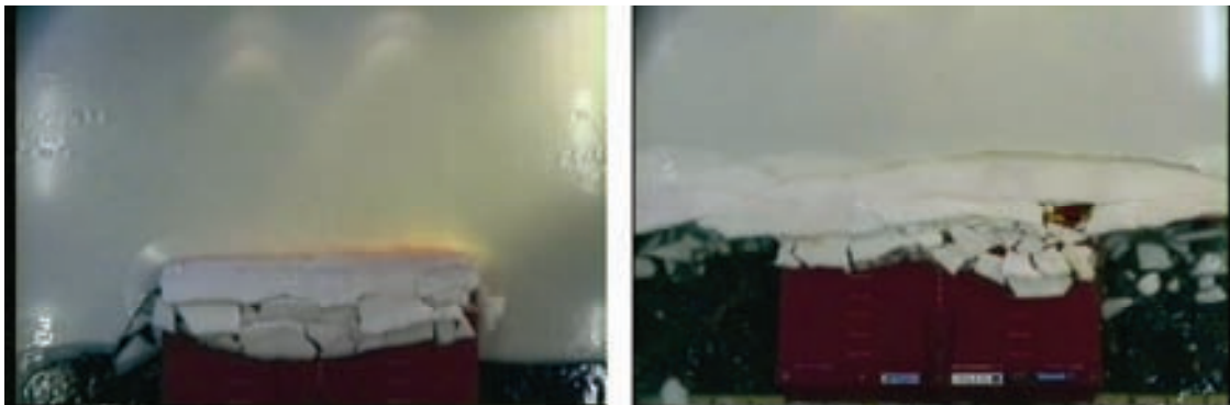
Figure 2.5.5. Top-view of initial ice breaking on the narrow SIB base structure (left) and the SIB base structure with side panels attached (right).
