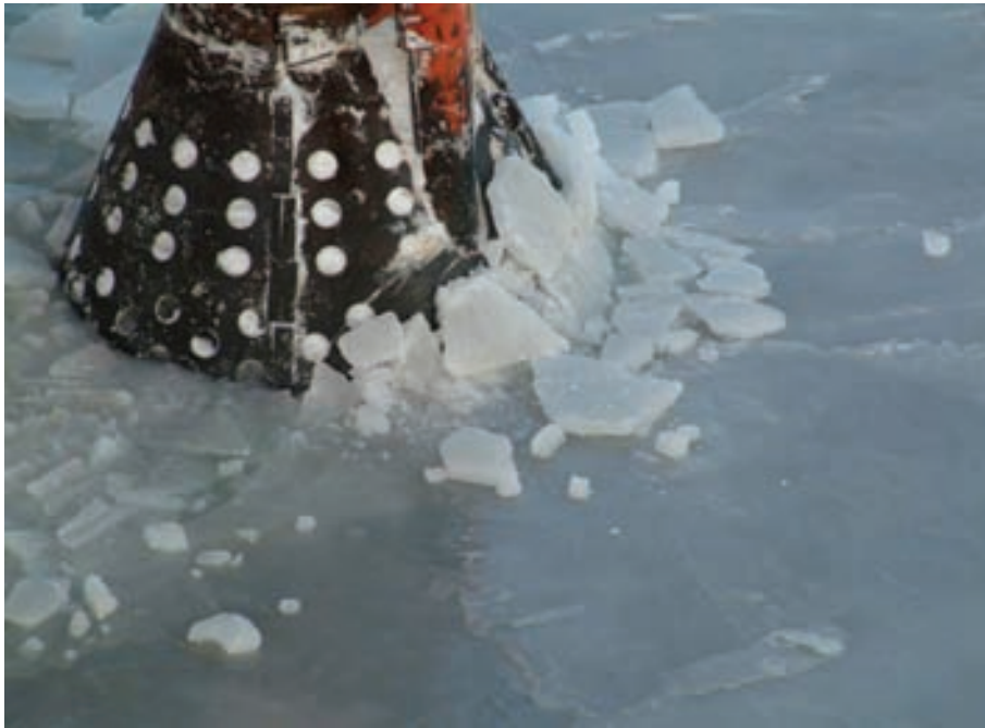
Figure 3.2.3. Ice interaction on a narrow cone in the Bohai Bay.
