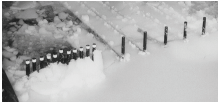
Figure 3.3.16. Differences in ice failure mode for l = 2D (left) and l = 8D (right) observed during physical model testing.
