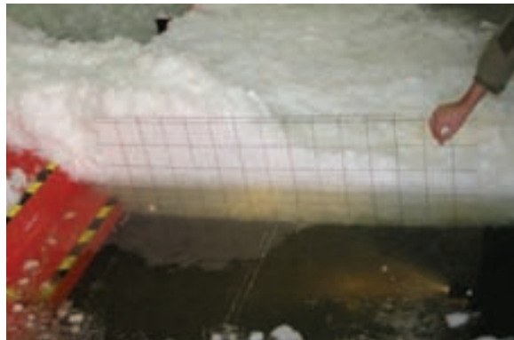
Figure 2.4.6. Physical inspection of the ice rubble pile in the centre.
