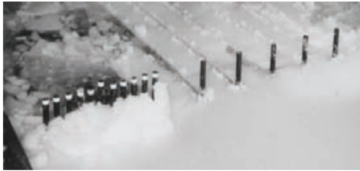
Figure 2.6.7. Pile arrangements ① and ② during the first test run showing the difference in failure mode as a dependence on the pile to pile spacing.
