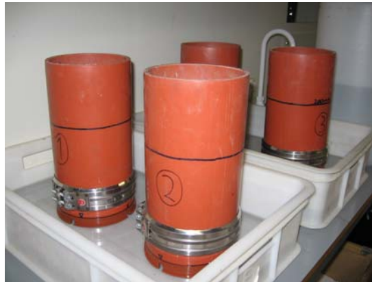
Figure 13. Sample setup for Tube Suction test during ten days of water absorption (Uthus, 2007a)
