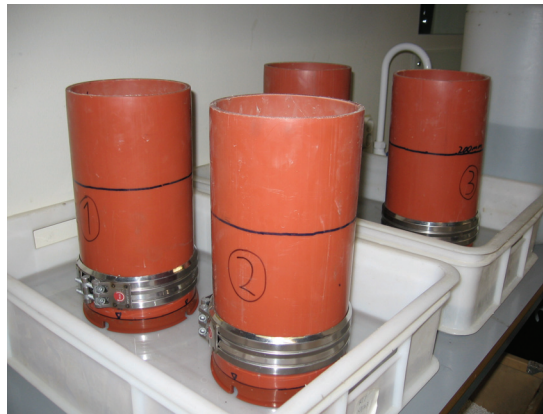
FIGURE 2. Sample setup during ten days of water absorption
