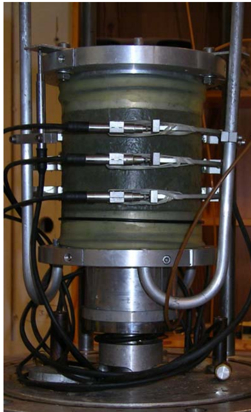
Figure 6. Instrumented triaxial sample (Dongmo-Engeland, 2005)
