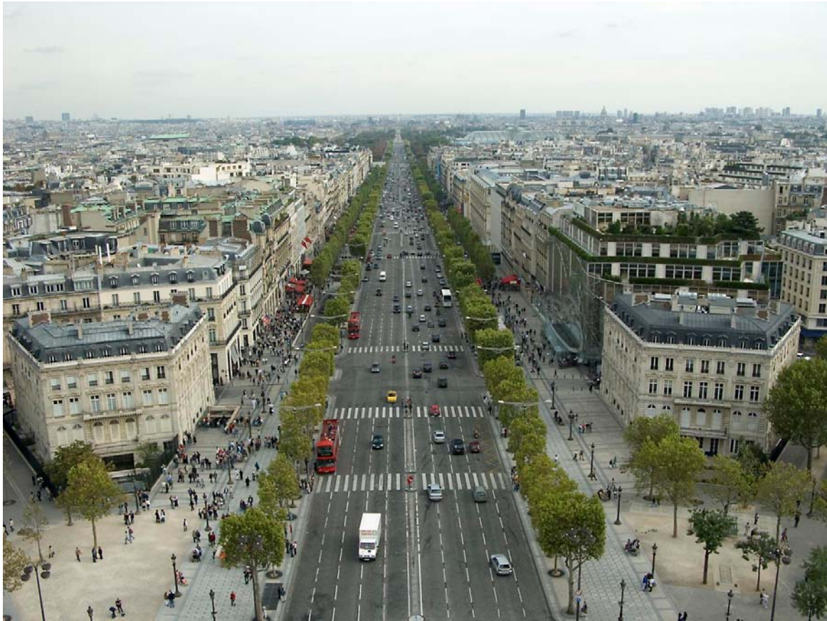
Figure 10.19: Avenue Champs-Élysées a ten lane avenue with a motorized traffic volume of approximately 125 000 AADT
