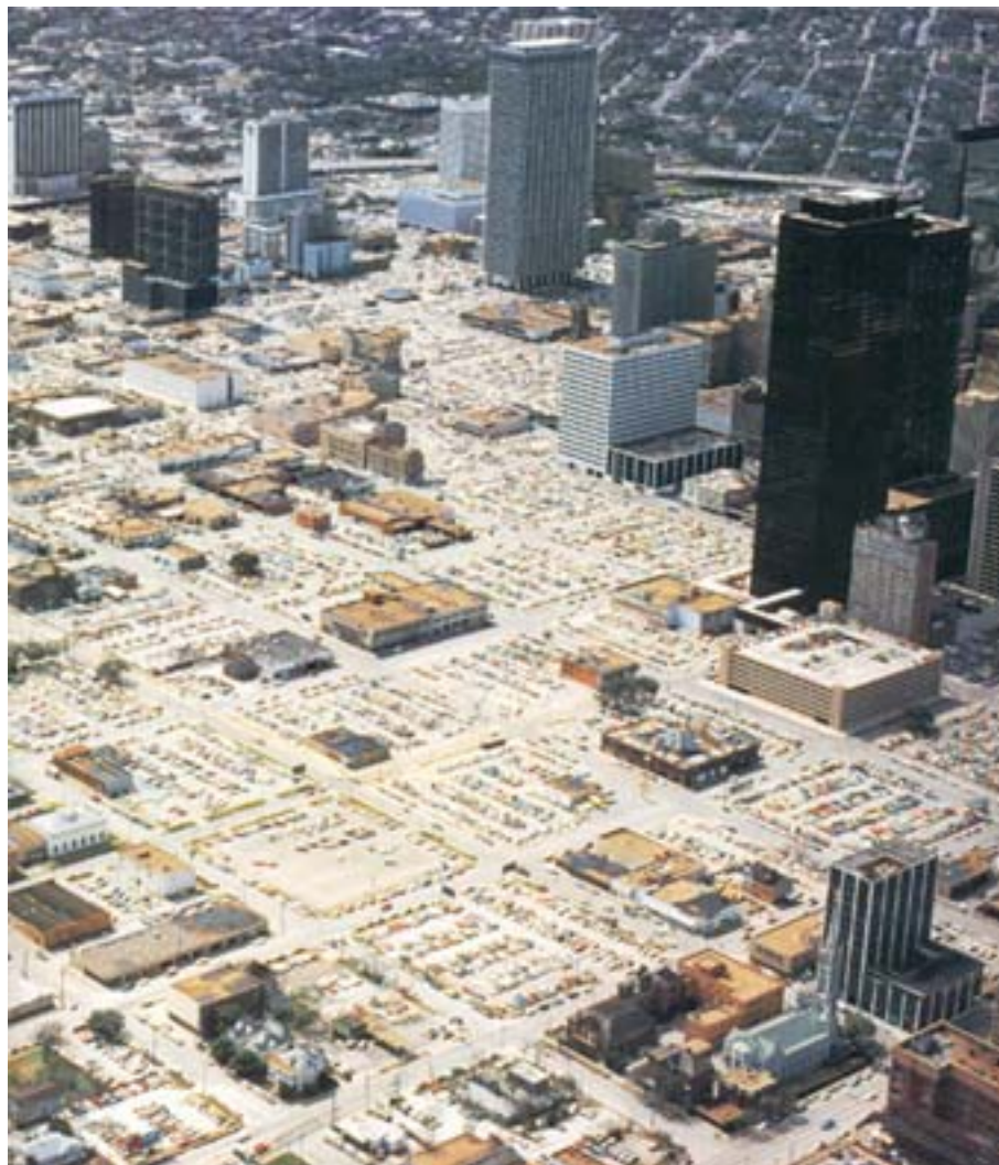
Figure 1.12: Houston, Texas has become an automobile-oriented city to the extreme. The historical street is totally absent leaving the city derelict and inhuman. 70% of the central business district is taken up by roadways and parking.
