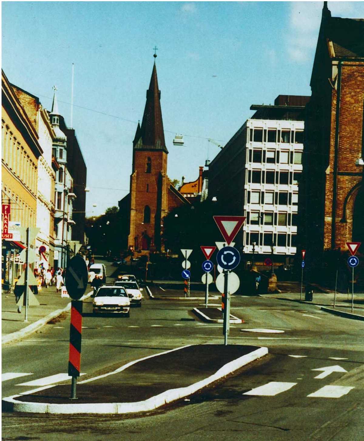
Figure 1.11: Akersgata, Oslo 2005. A new traffic system necessitates the establishment of two roundabouts, so inconspicuous that 21 traffic signs have to announce their presence, ignoring the original architectural order and harmony of the street
