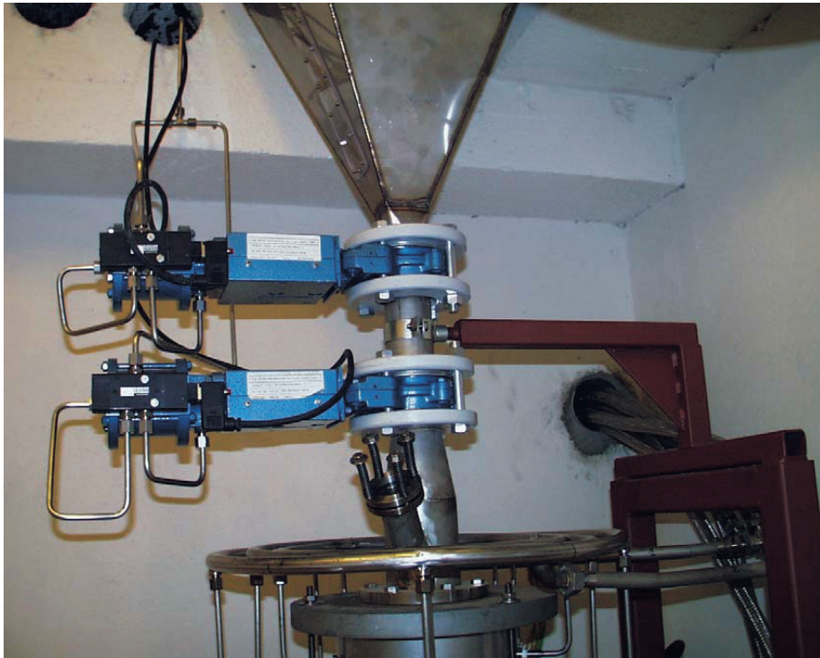
Figure A.3: Biomass feeding system
