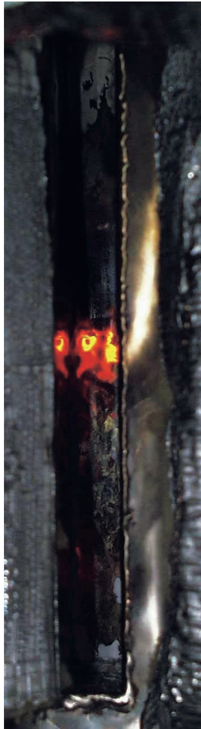
Figure A.6: Flaming pyrolysis inside the gasifier
