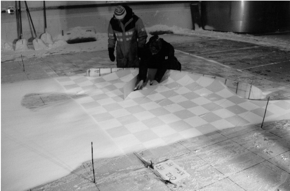
Figure 4.2 Snow depth measurements by surface tracing on a paper sheet in the Jules Verne Climatic Wind Tunnel.
