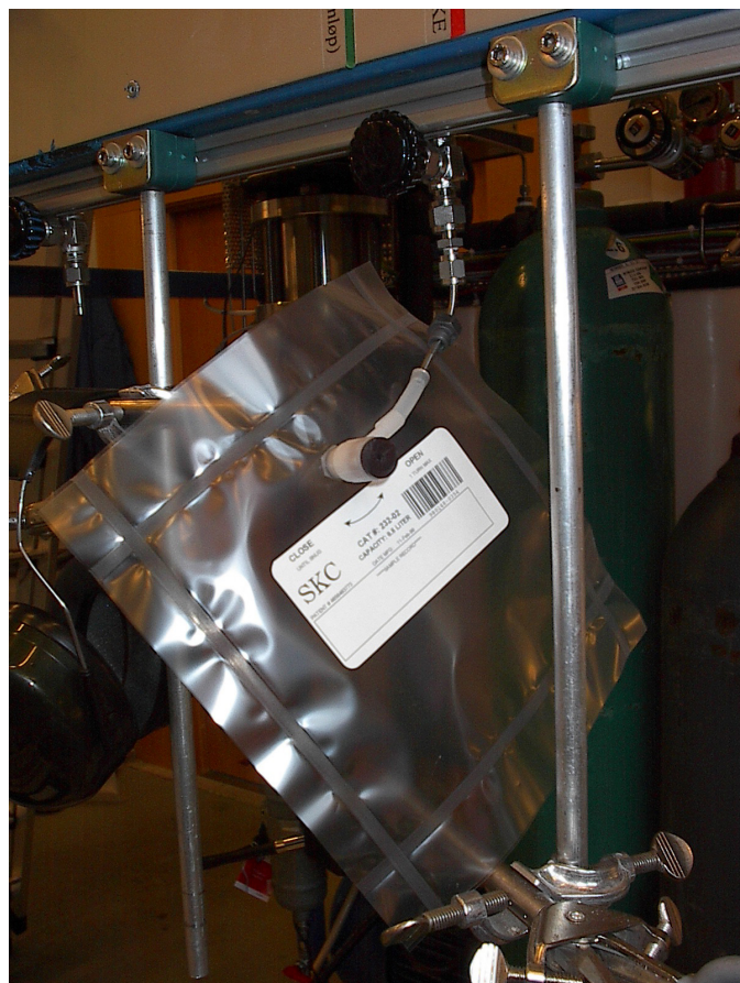
Figure 9-14 Gas sampling on wetted wall column
